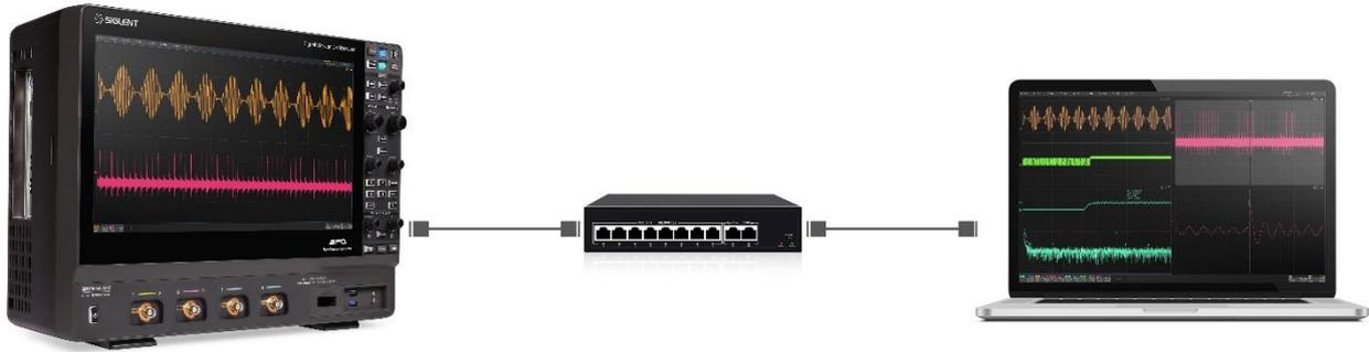
In this scenario, SigScopeLab only controls remote acquisition and does not control remote analysis and measurement. SigScopeLab fetches waveform data from the remote device online after controlling the acquisition, and then performs local data analysis. Please refer to the following steps:
