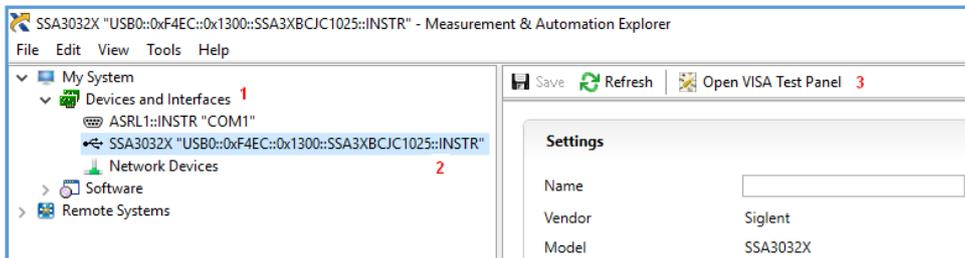
4. Click “Open VISA Test Panel” option button, and then the following Interface will appear. Then click the “Input/Output” option button and click the “Query” option button in order to view the Read operation information.
