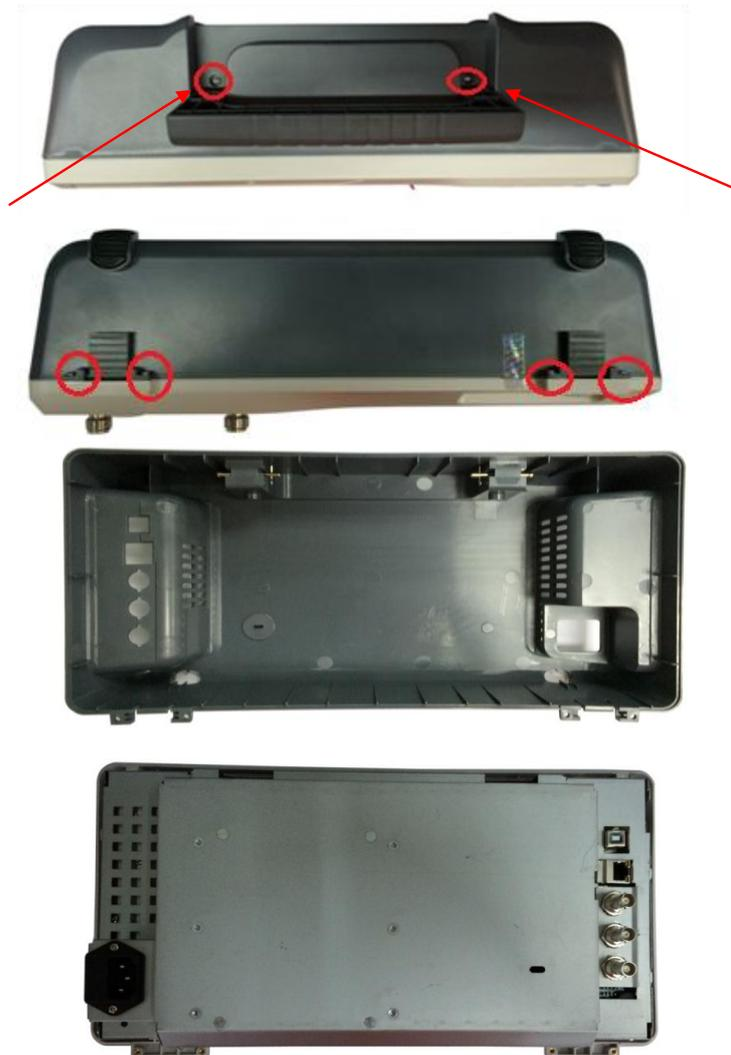
Figure 4-1 Removing the Rear Panel Screws
