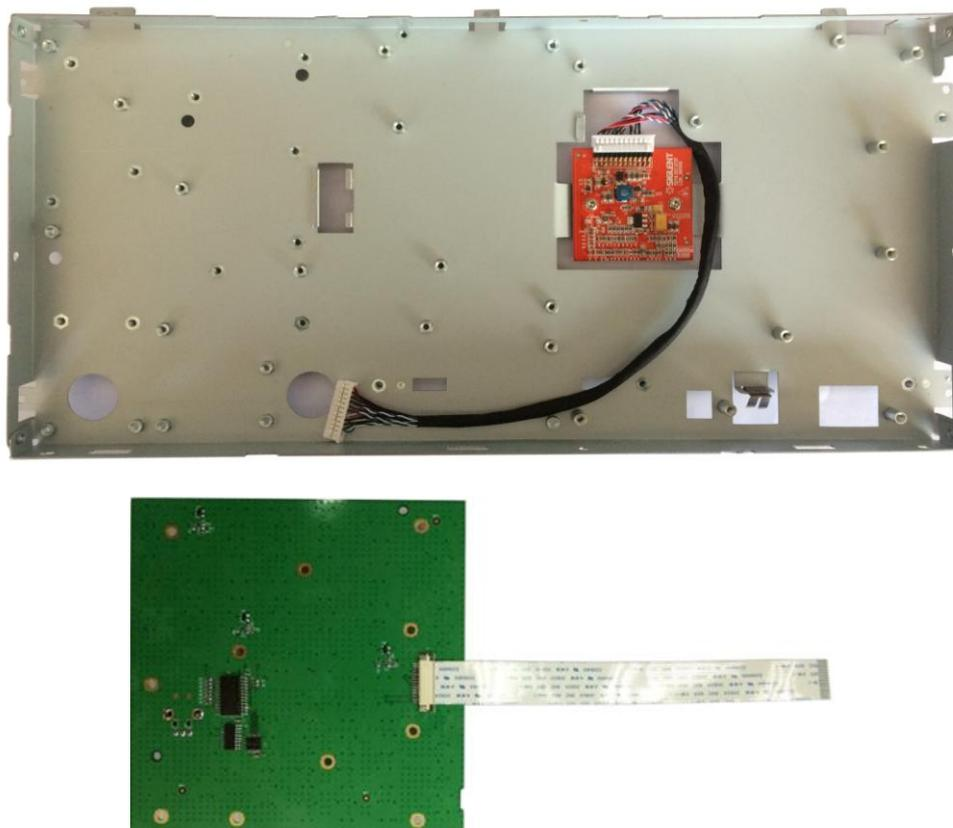
Figure 4-5 Removing the LCD and keyboard
