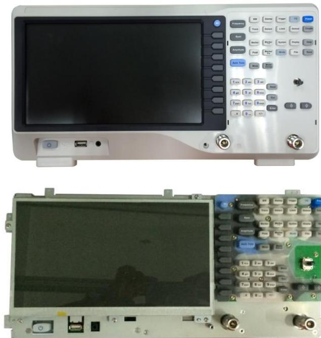
Figure 4-2 Removing the front panel
