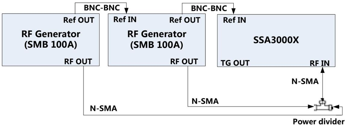
Figure 3-5 TOI verification connections
