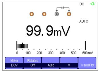
Figure 3-2 DC Voltage Measurement
