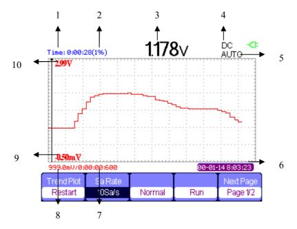
Figure 4-12 Multimeter Trend Plot User Interface
