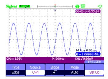
Figure 2-39 Signal Rise Trigger Menu
