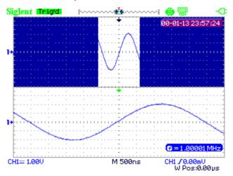
Figure 2-21 Delay Scan Waveform
