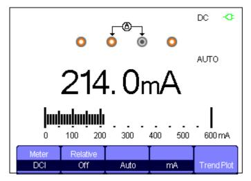
Figure 3-8 DC Current "mA" Measurement
