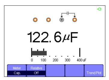
**Figure 3-7 Capacitance Measurement**
