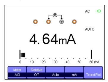
Figure 3-10 AC Current "mA" Measurement
