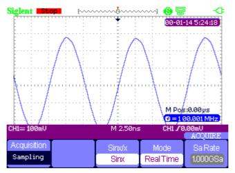
Figure 2-9 Sinx Interpolation
