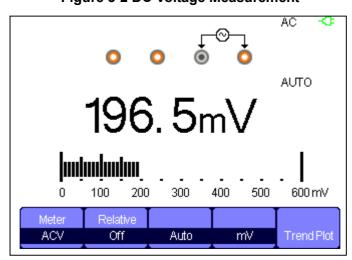
Figure 3-3 AC Voltage Measurement
