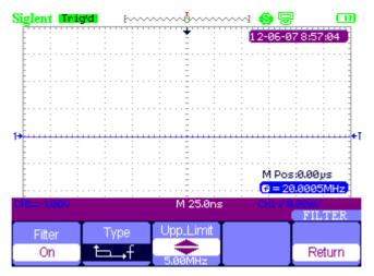
Figure 2-6 After Turn On the Digital Filter
