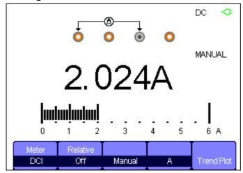
Figure 3-9 DC Current "A" Measurement
