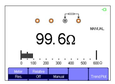
**Figure 3-4 Resistance Measurement**
