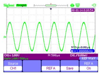
Figure 2-25 Reference Waveform
