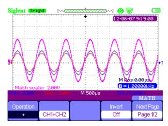
Figure 2-16 Result of Two Waveforms Add
