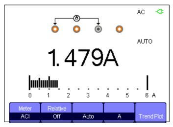
Figure 3-11 AC Current "A" Measurement
