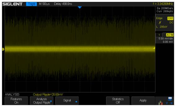
Figure 123: Perform Output Ripple Analysis
