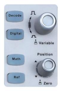
Press this button to open decode menu. Decode is an optional function. SDS2000X supports two serial buses including 1 and 2 for analog signal decoding. The protocols include I2C, SPI, UART/RS232, CAN and LIN.
