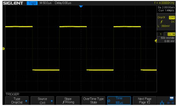
Figure 32: State DropOut Trigger
