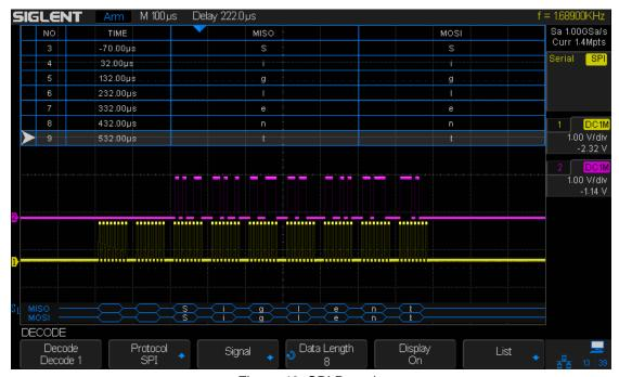
Figure 46: SPI Decode
