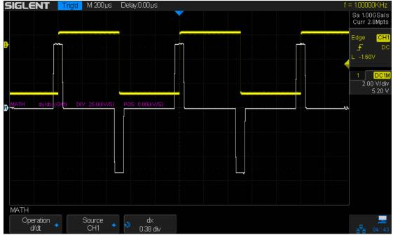
Figure 69: Differential Function Operation
