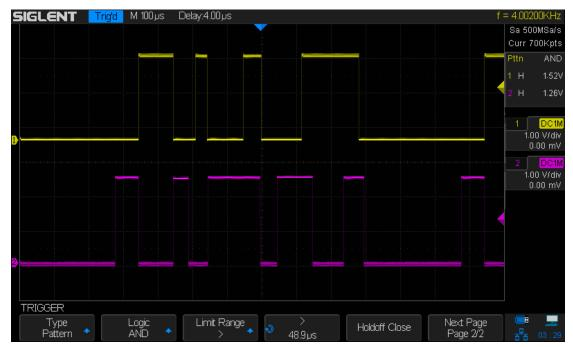
Figure 34: Pattern Trigger
