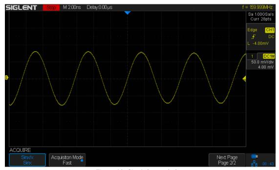
Figure 13: Sinx/x Interpolation
