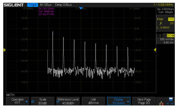
Figure 68 FFT Waveform in Exclusive Mode
