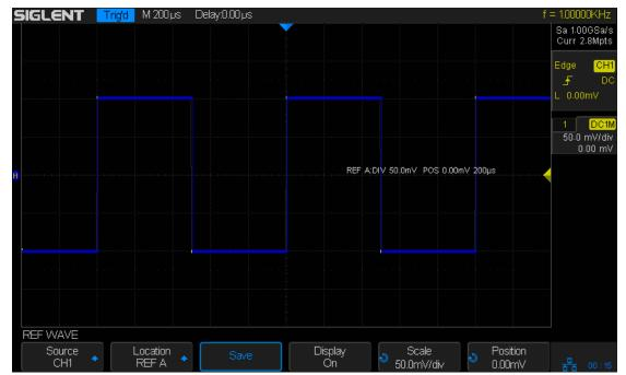
Figure 65: Reference Waveform
