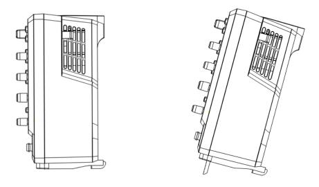
Figure 3: Adjust the Supporting Legs
