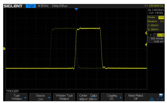
Figure 29: Relative Window Trigger
