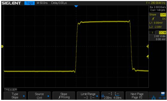
Figure 25: Slope Trigger
