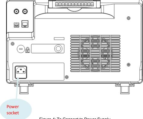
Figure 4: To Connect to Power Supply
