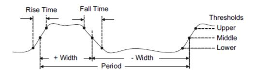
Figure 77: Time Measurements
