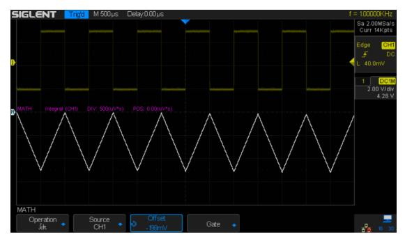
Figure 71: Integral with Offset
