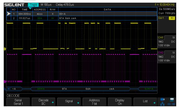
Figure 39: IIC Decode Result
