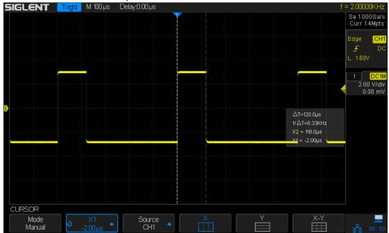
Figure 73: Measure Pulse Width
