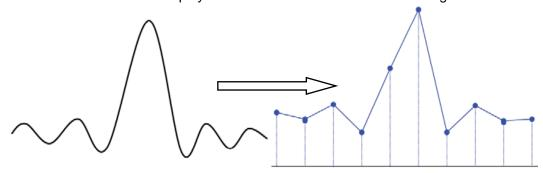
2. Waveform Aliasing: when the sample rate is lower than twice the actual signal frequency (Nyquist Frequency), the frequency of the waveform rebuilt from the sample data is lower than the actual signal frequency. The most common aliasing is the jitter on fast edge.
