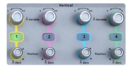
Analog input channels. The four channels are marked by different colors which are also used to mark both the waveforms on the screen and the channel input connectors. Press channel button to open the corresponding channel and press again to turn it off.
