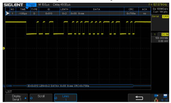
Figure 54: CAN Decode
