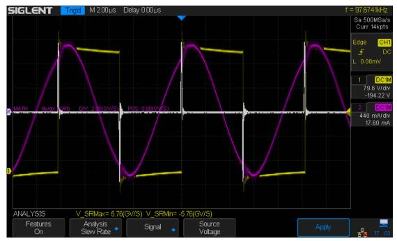
Figure 117: Perform Slew Rate Analysis
