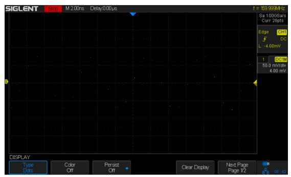
Figure 11: Display Type Set to Dots
