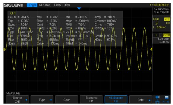
Figure 80: All Parameters Measurement
