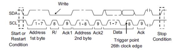
Data Length — When the SDA data length is equal to the value of Byte Length
