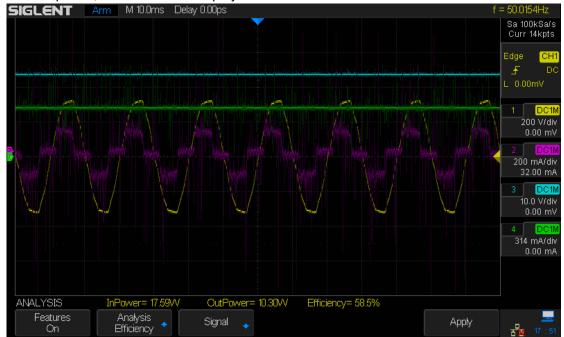
Figure 134: Perform Efficiency Analysis
