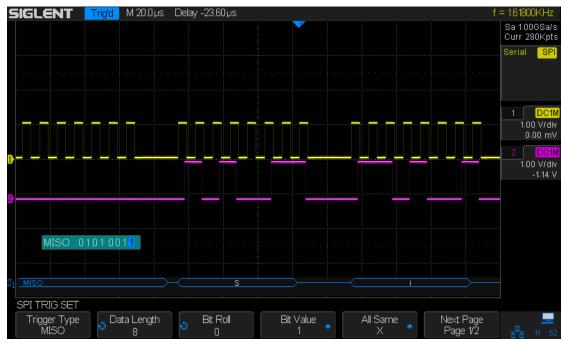
Figure 45: SPI Trigger
