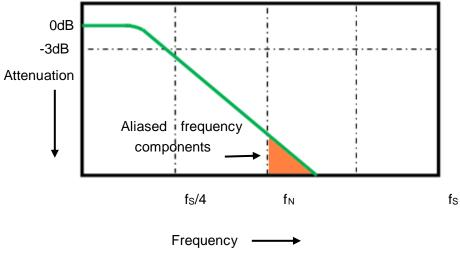
Limiting oscilloscope bandwidth ( $f_{BW}$ ) to ½ the sample rate ( $f_{S}/4$ ) reduces frequency components above the Nyquist frequency ( $f_{N}$ ).
