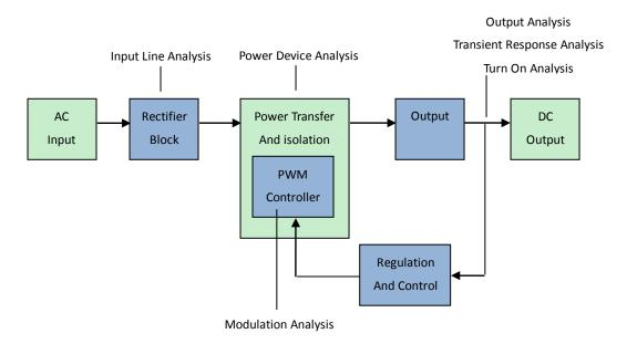
Switch-Mode Power Supply (SMPS) Block Diagram and Types of Measurements
