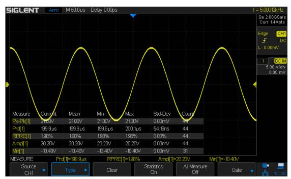
Figure 79: Add the Measurement
