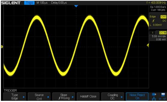
Figure 23: Turn on Noise Reject
