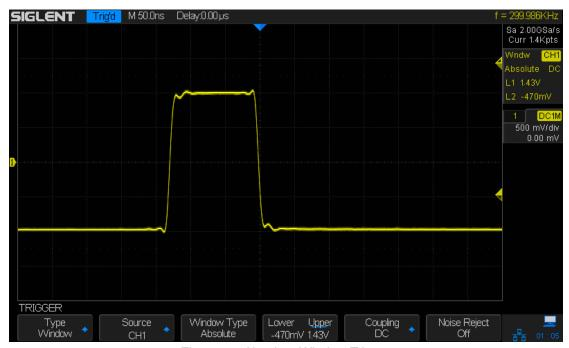
Figure 28: Absolute Window Trigger
