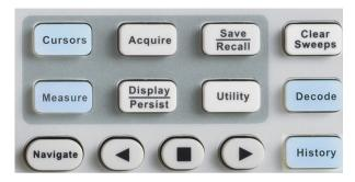
Cursors Press the button to open the cursor function. It provides manual and track cursor mode.
