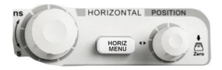
HORIZ HORIZ: Press the button to open horizontal control menu under which you can turn on/off the delay sweep function.
