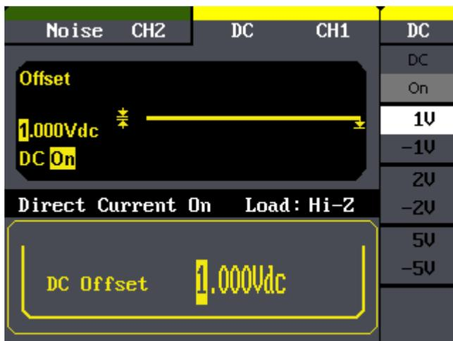
You can enter any dc voltage from -10Vdc to +10Vdc (Only Channel 1).
