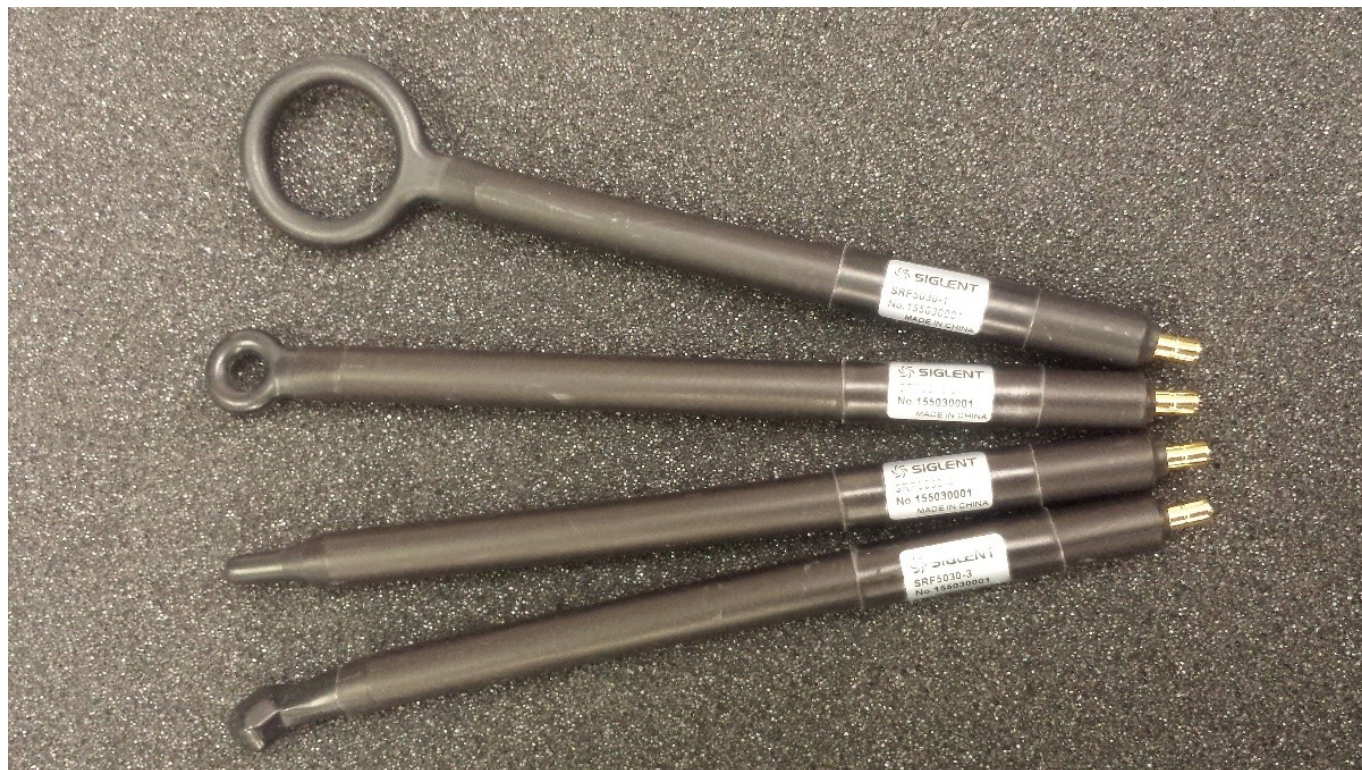
Figure 5: SIGLENT SRF5030 near-field probe kit.
