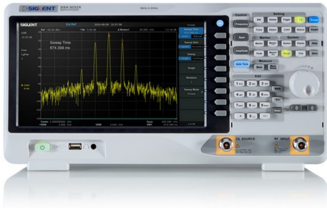
Figure 3: A SIGLENT SSA3021X 2.1 GHz spectrum analyzer.
