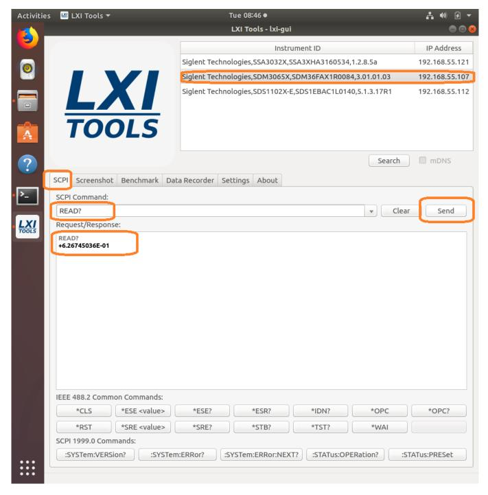
NOTE: The specific commands that can be used are available in the instrument programming guide. Check out the specific instrument documentation for more details.
