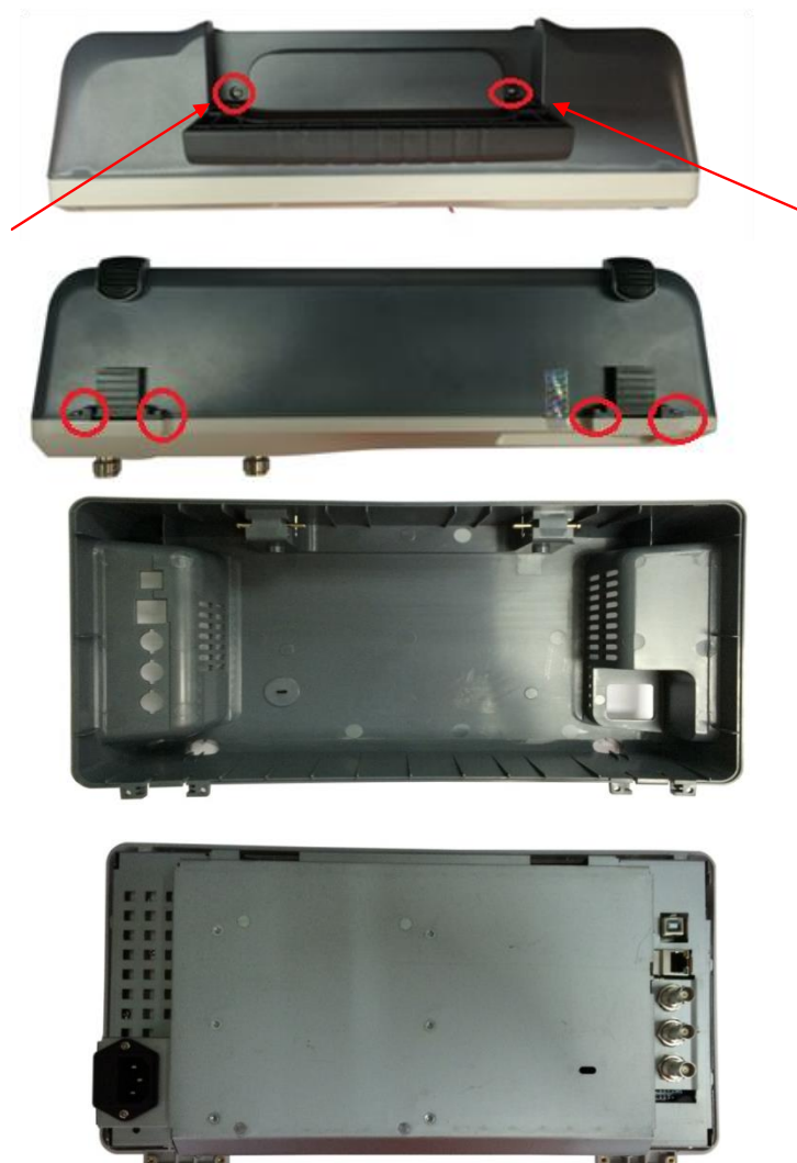
Figure 4-1 Removing the Rear Panel Screws
