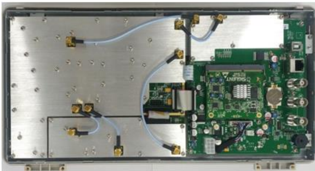
Figure 4-4 View of front panel subassembly with main board
