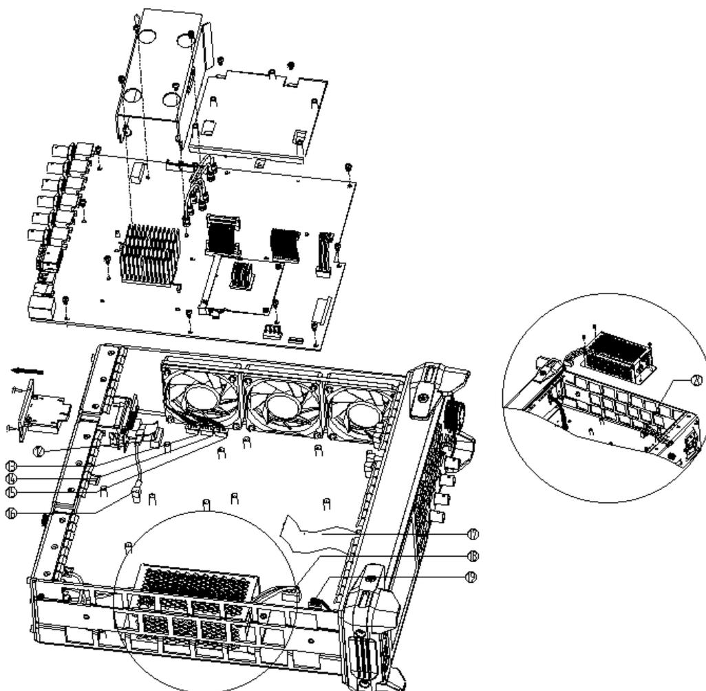
Figure 5-3 Disassemble the Main Board
