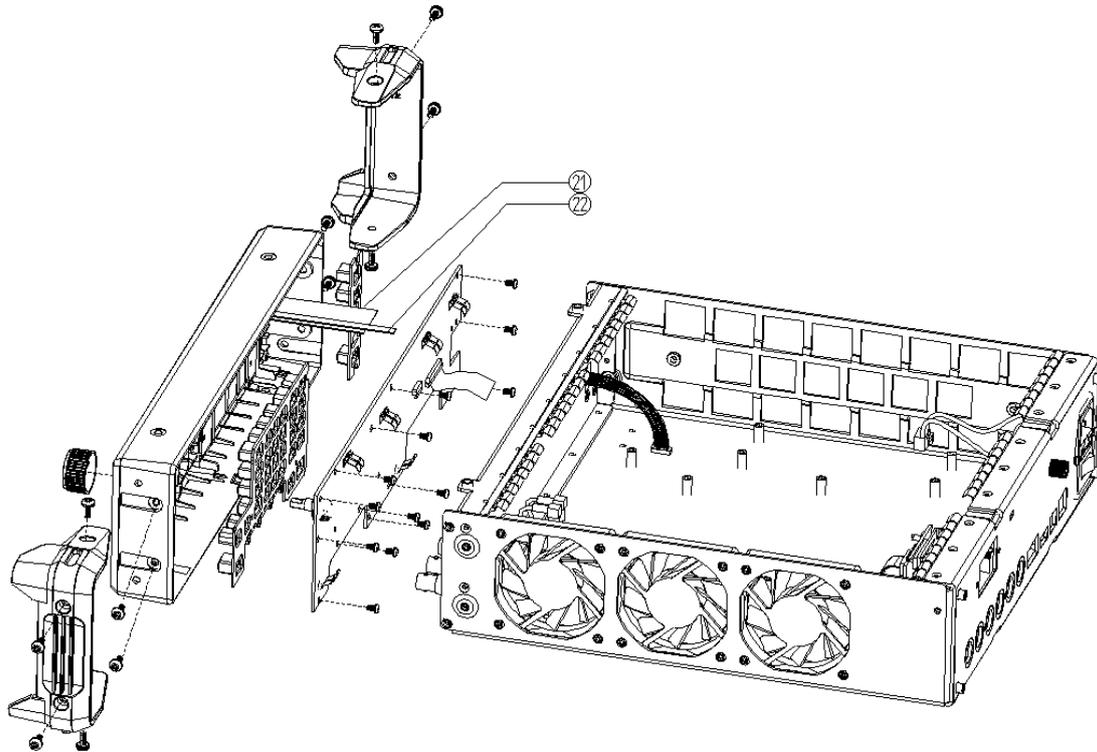
Figure 5-4 Disassemble the Front Cabinet
