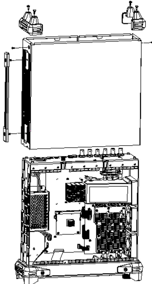
Figure 5-1 Disassemble the Metal Shell
