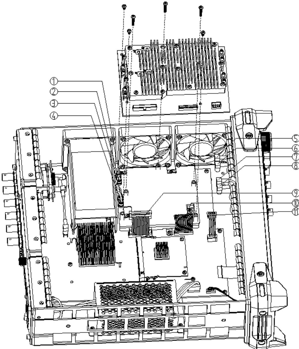
Figure 5-2 Disassemble the Channel Board
