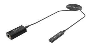
The SAP5000D differential probe is provided with 5GHz bandwidth, 80 ps rise time, 400 fF differential input capacitance, and 10:1 attenuation ratio
