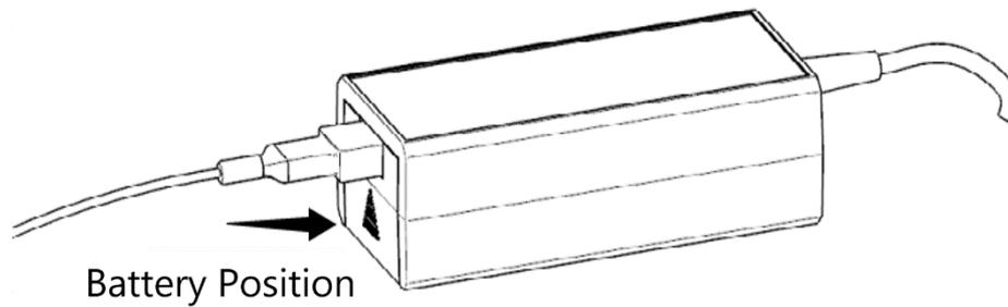
The standard configuration contains two 7.4 V/950 mAh lithium batteries. The battery installation position is shown in the above figure. In this design, after inserting the attenuator, the attenuator plays a limiting role and the battery cannot be removed. If you need to remove the battery for charging, refer to the following steps:
