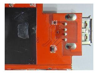
4. Solder the tip of the head to the test points on the circuit board.
