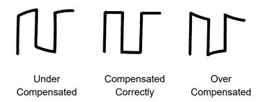
3) Adjust the probe until the waveform matches the "Compensated Correctly" waveform above.
