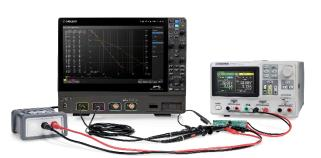
The oscilloscope can control the Built-in waveform generator, SIGLENT isolated USB AWG module or a stand-alone SIGLENT SDG generator, to scan the amplitude and phasefrequency response of the DUT, and display the data as a Bode Plot. This makes it possible to replace expensive network analyzers in some applications
