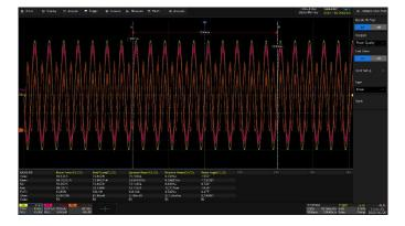
The Power Analysis option provides a full suite of power measurements and analysis, which greatly improve the measurement efficiency in switching power supplies and power devices design
