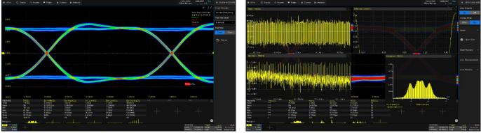
Supports eye diagram and jitter analysis/measurement. It can automatically extract the embedded reference clock from serial data and create the eye diagram. Measurement on multiple eye/jitter parameters is provided. Mask test on eye diagrams is supported
