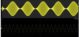
Using hardware-based Zoom technique and record length of up to 1 Gpts, users can select a slower timebase without compromising the sample rate, and then quickly zoom in to focus on the area of interest
