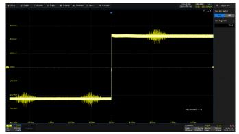
Segmented memory collection will store the waveform into multiple memory segments (up to 124,000) and each segment will store a triggered waveform as well the dead time information. The interval between segments can be as small as 0.9  $\mu$ s. All of the segments can be played back using the History function
