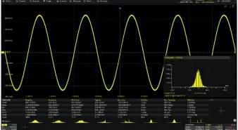
Statistics show the current value, maximum value, minimum value, standard deviation, and mean value of up to 12 parameters simultaneously. A histogram is available to show the probability distribution of a parameter. Trend and Track are available to show the parameter value vs. time.
