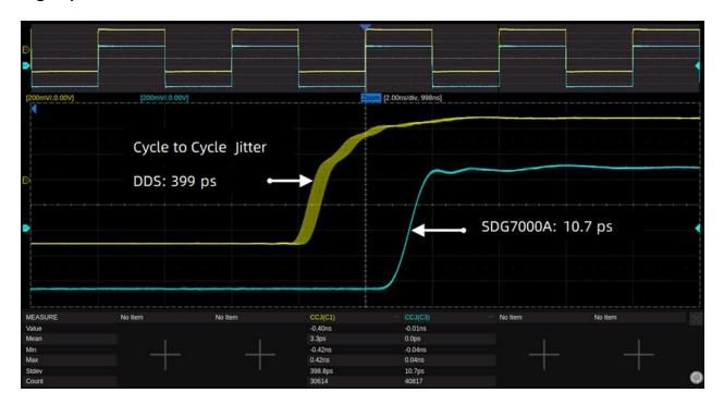
**Low jitter** When a Square/Pulse waveform is generated by traditional DDS, there can be additional jitter if the sample rate is not an integer-related multiple of the output frequency. EasyPulse technology successfully overcomes this weakness in DDS designs and helps to produce low jitter Square/Pulse waveforms.
