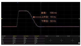
**Flexible edge** Adjustable fine step resolution to 100 ps. The minimum edge is 500 ps and can be generated at any frequency. The rising/ falling edge can be set respectively and can be used to generate asymmetric pulse.
