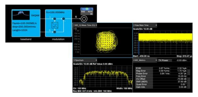
The SDG7000A can generate common modulation types of IQ signals, such as ASK, FSK, PSK, QAM. With the innovative resampling technology, excellent EVM performance can be obtained at any symbol rate between 250 S/s  $\sim$  500 MS/s. The built-in digital quadrature modulator can modulate the carrier of the IQ signal to any frequency between 0 Hz $\sim$ 1 GHz. The EasyIQ software can be used to generate and edit various types of IQ signals.
