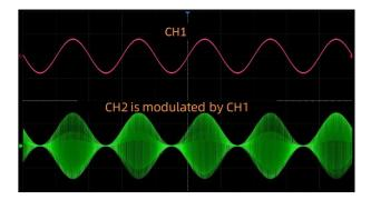
**Channel Modulation** One channel can modulate the other without external connections. This feature provides an easy method for complex modulation waveform creation. The modulating wave channel can be directly output and compared with the modulated signal.
