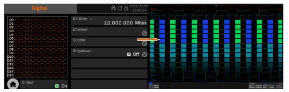
Purchase the corresponding digital bus kit to get 16-channel LVTTL or LVDS output with a bit rate of 1  $\mu$ bps ~ 1 Gbps. Combine the digital bus with the analog channels to realize mixed-signal outputs.
