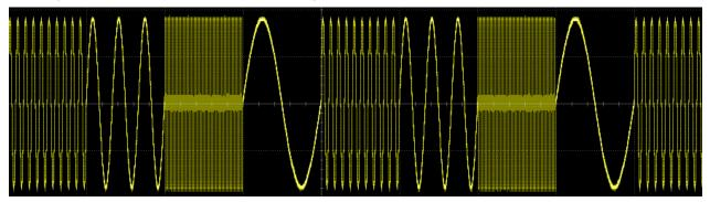
**Multi pulse** Supports multi pulse output. The positive and negative pulse widths of each pulse can be individually edited and set through EasywaveX tools.
