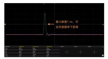
**High speed** The minimum 1 ns pulse width, can be generated at any frequency. The pulse width can be finely adjusted in steps of 10 ps.
