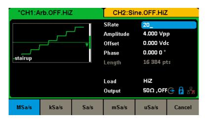
Figure 2-20 Setting the Sampling Rate
