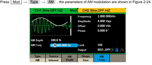
Figure 2-24 Setting Interface of AM Modulation
