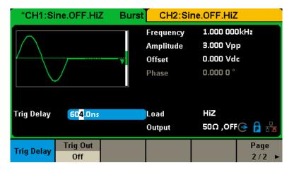
Figure 2-39 N-Cycle Burst Interface (Page 2/2)
