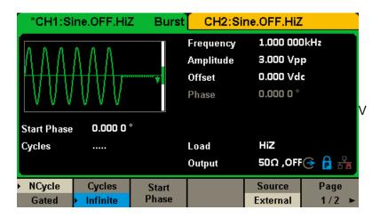
Figure 2-40 Infinite Burst Interface
