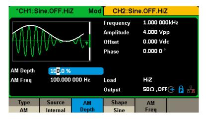
Figure 1-14 Modulation Display Interface
