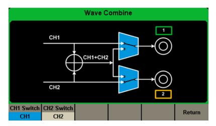
Figure 2-71 Waveforms Combining Interface
