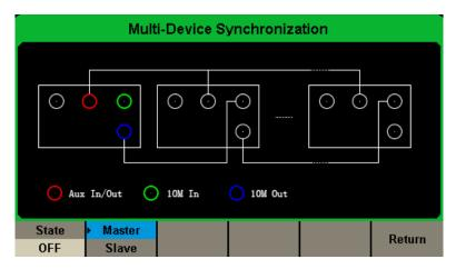
Figure 2-86 Multi-Device Sync Interface
