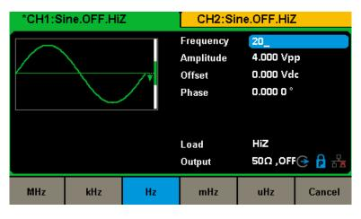
Figure 2-2 Setting the Frequency
