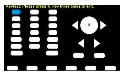
Figure 2-62 Key Test Interface
