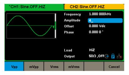
Figure 2-3 Setting the Amplitude
