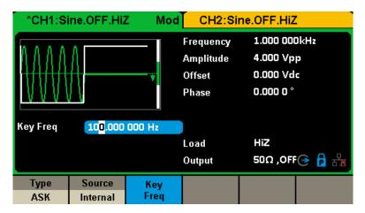
Figure 2-29 Setting Interface of ASK Modulation
