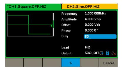
Figure 2-7 Setting the Duty Cycle
