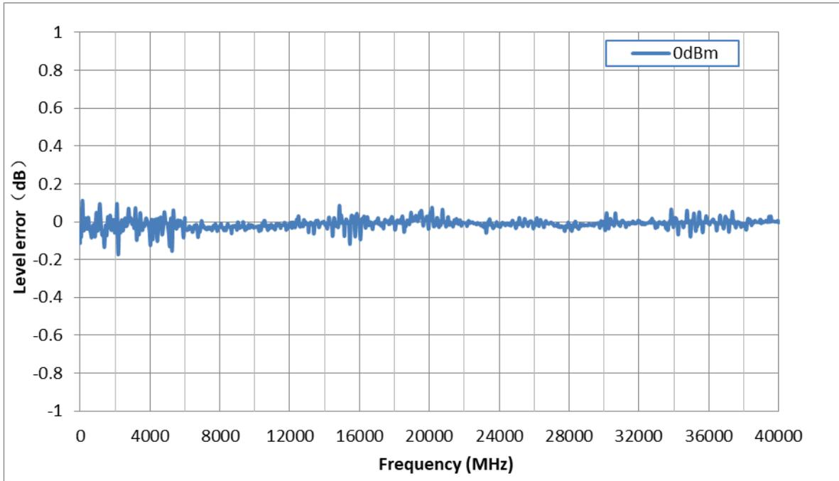
Measured level error versus frequency, Level = - 20 dBm
