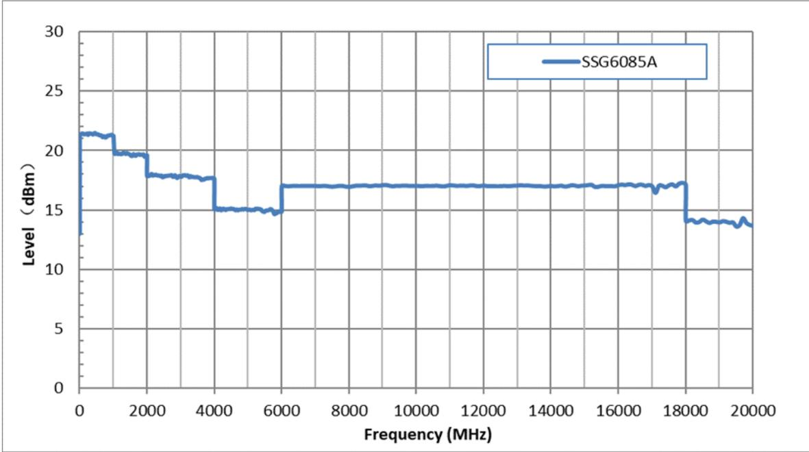
Measured level error versus frequency, Level = 10 dBm
