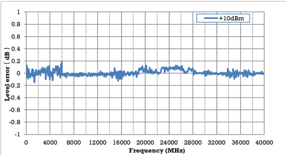
Measured level error versus frequency, Level = 0 dBm
