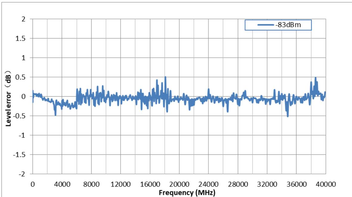
Measured level error versus frequency, Level = - 120 dBm
