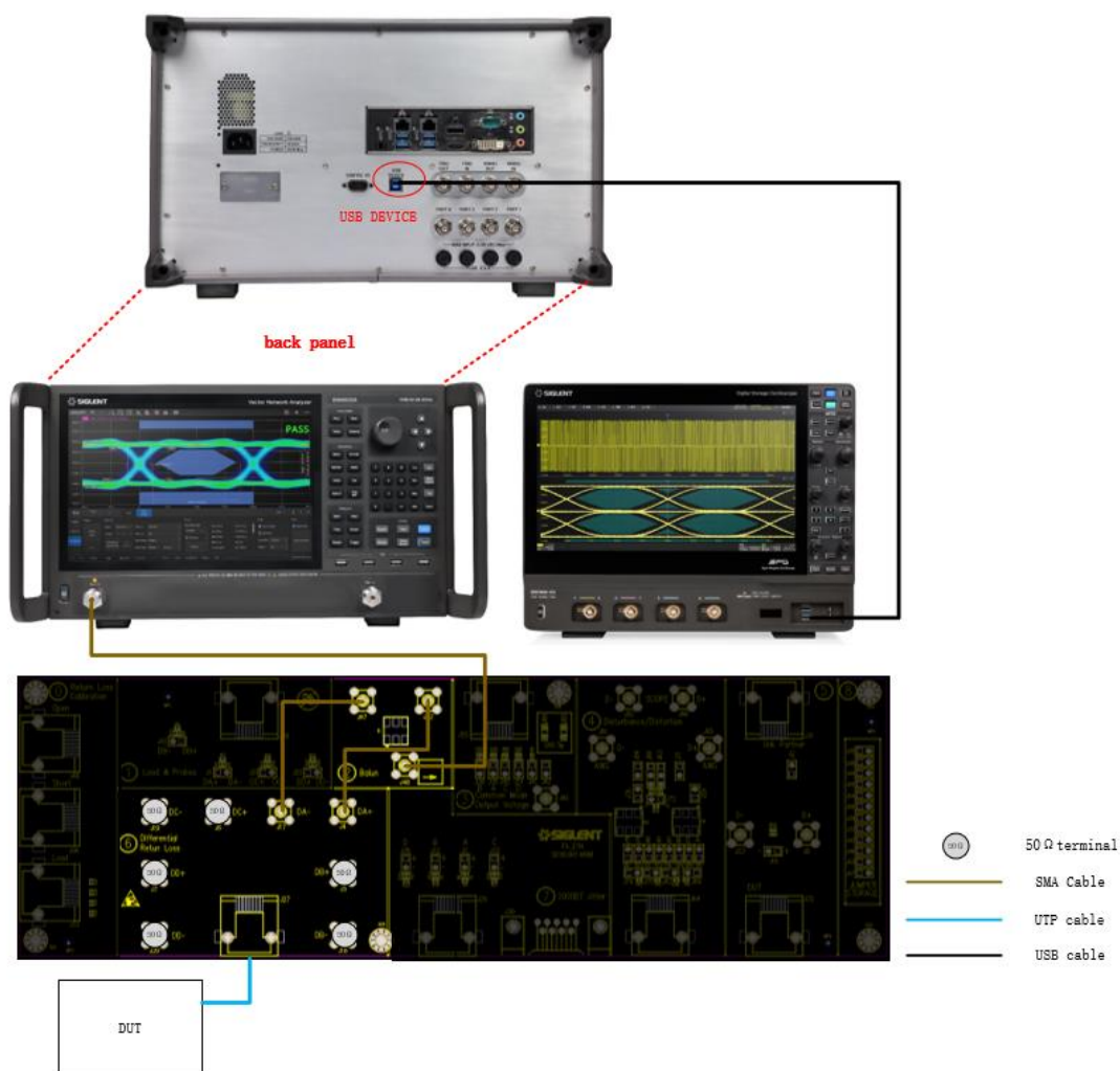
Figure 6-18 Transmitter Return Loss Test Environment
