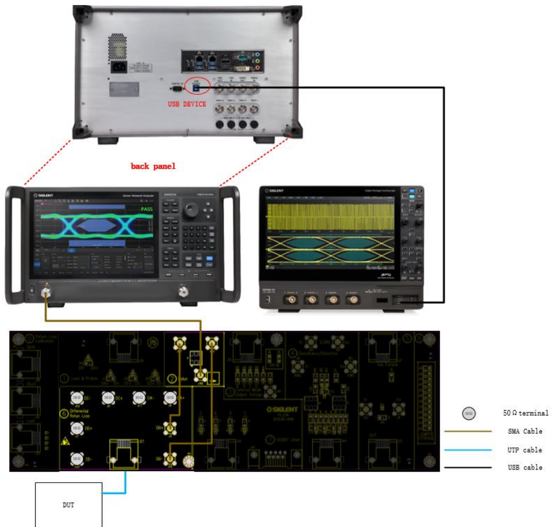
Figure 6-22 Receiver return loss test connection
