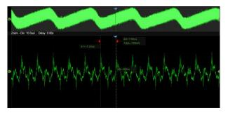
Using a hardware-based Zoom technique and record length of up to 500 Mpts, users can select a slower timebase without compromising the sample rate, and then quickly zoom in to focus on the area of interest.
