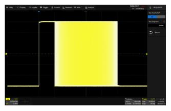
Segmented memory collection will store the waveform into multiple memory segments (up to 80,000) and each segment will store a triggered waveform as well as the dead time information. The interval between segments can be as small as 1.3µs. All of the segments can be played back using the History function.
