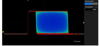
Segmented memory collection will store the waveform into multiple memory segments (up to 100,000) and each segment will store a triggered waveform as well the dead time information. The interval between segments can be as small as 2  $\mu$ s. All of the segments can be played back using the History function
