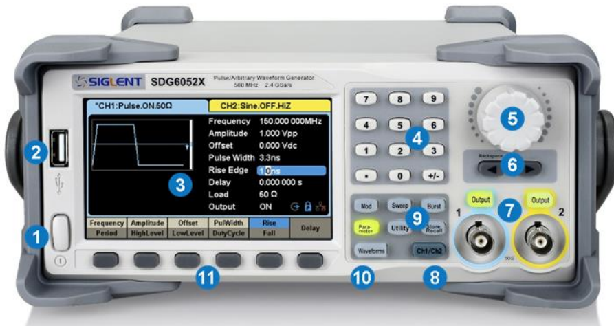
Figure 2 SDG6000X Front Panel
