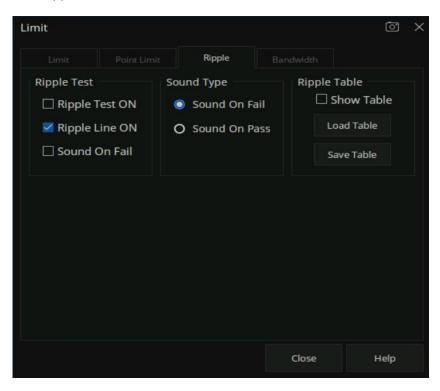
Figure 7-10 Ripple test setting interface
