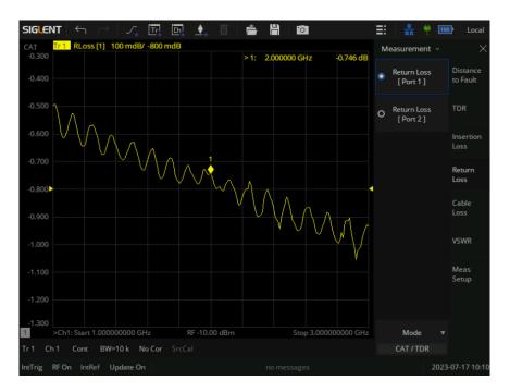
Figure 11-7 Return loss measurement interface
