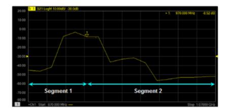
Figure 5-3 Use X-axis point spacing
