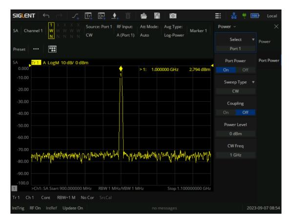
Figure 9-8 Press the [Power] key to enter the source's setting menu
