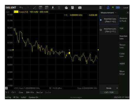
Figure 11-6 Insertion loss measurement interface
