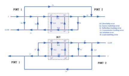
Figure 6-25 Error model diagram
