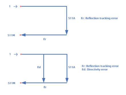
Figure 6-22 Schematic diagram
