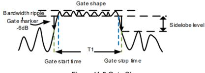
The parameters of gating function are defined as shown in the following figure:
