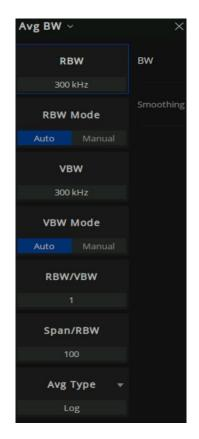
Figure 9-4 Spectrum analysis signal processing setup menu
