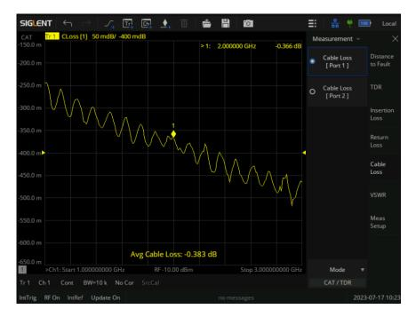
Figure 11-8 Cable loss measurement interface
