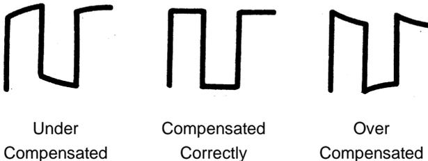
3. Use a nonmetallic flat-head screwdriver to adjust the low-frequency compensation adjustment hole on the probe until the waveform matches the “Compensated Correctly” waveform above.
