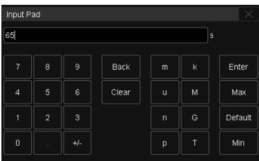
To use the operation of setting “deskew” of the channel as an example: If the expected value is 65 ns, input “65” on the virtual keypad, and then choose the unit **n** to complete the operation. On the virtual keypad, touching the button **Max**, **Min**, and **Default** quickly sets the parameter to its maximum, minimum and default values.
