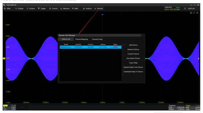
Step 3: Click to select the item of device list to be connected, then continue to click *Connect Device*. After the device status is updated to *online*, local analysis can be performed with the waveform data acquired in real time from the device.
