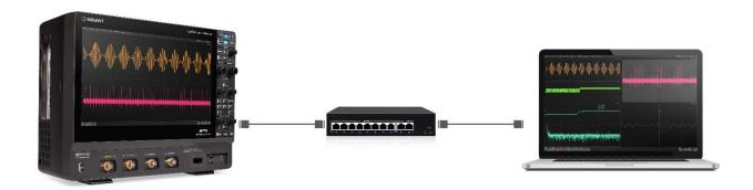
In this scenario, SigScopeLab only controls remote acquisition and does not control remote analysis and measurement. SigScopeLab fetchs waveform data from the remote device online after controlling the acquisition, and then performs local data analysis. Please refer to the following steps:
