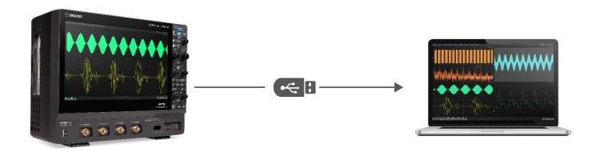
Firstly, export binary waveform files from any SDS device and place them in any computer accessible location via a USB flash drive or network server.
