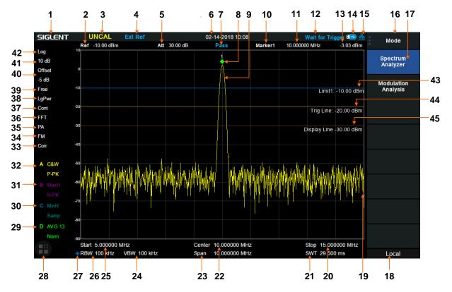
Figure 12 User Interface of Spectrum Analyzer Mode
