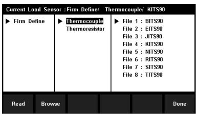
Diagram 3-14 Select the Type of Thermocouple
