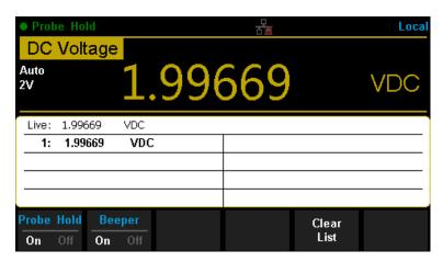
Diagram 2-68 Hold Measurement Function Interface
