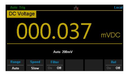
Diagram 2-4 DC Voltage Measurement Interface
