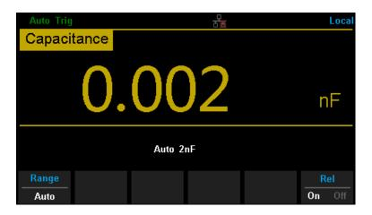
Diagram 2-17 Capacitance Measurement Interface
