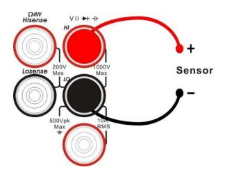
Diagram 2-28 Sketch Map for Measuring Temperature
