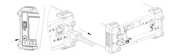
3 Press the connector button with your finger, and then insert the connecting line.
