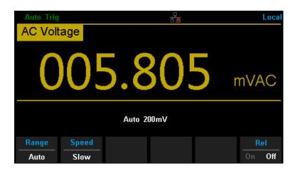
Diagram 2-8 AC Voltage Measurement Interface
