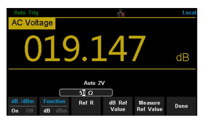
Diagram 3-8 Set the Parameters of dB
