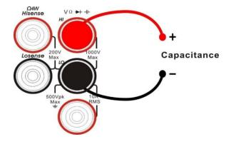
Diagram 2-18 Sketch Map for Measuring Capacitance
