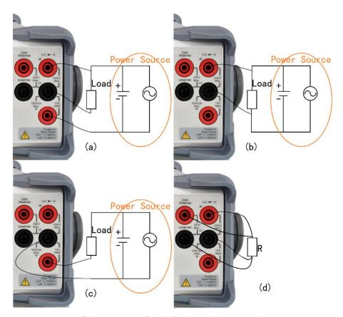
Diagram 2-39 Dual-display wiring example
