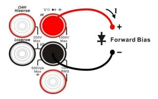
Diagram 2-26 Sketch Map for testing Diode
