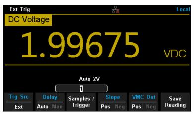
Diagram 2-55 Setting interface of Ext Trigger
