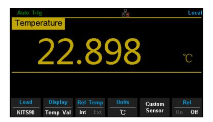
Diagram 2-27 Temperature Measurement Interface
