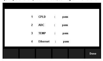
Diagram 2-50 Chip Test Interface
