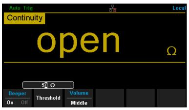
Diagram 2-37 Set Up the Short-circuit Resistance
