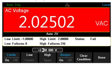
Diagram 3-12 Limits Test Result
