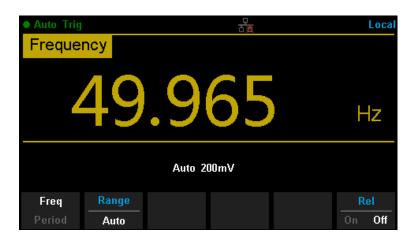
Diagram 2-19 Frequency Measurement Interface
