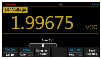
Diagram 2-54 Setting interface of Auto Trigger
