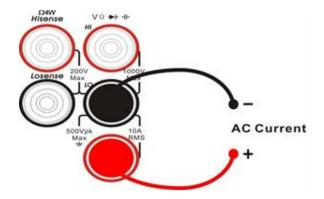
Diagram 2-12 Sketch Map for Measuring AC Current
