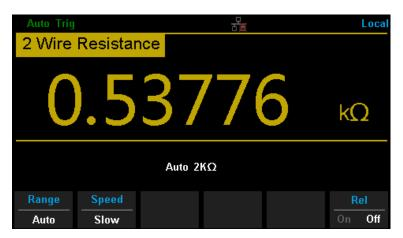
Diagram 3-3 Test Lead Impedance
