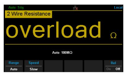
Diagram 2-13 2-Wire Resistance Measurement Interface
