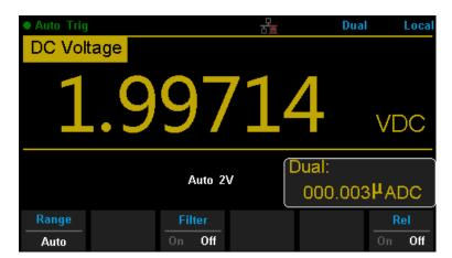
Diagram 2-38 Dual-display function Interface (Main DCV, Vice DCI)
