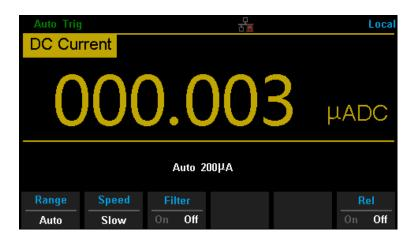
Diagram 2-6 DC Current Measurement Interface
