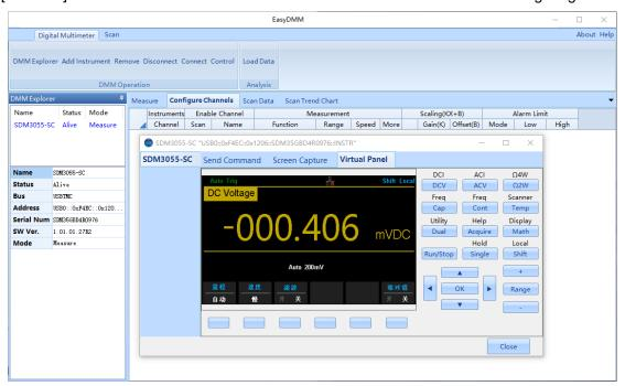
Diagram 3-19 The Main Interface of EasySDM
