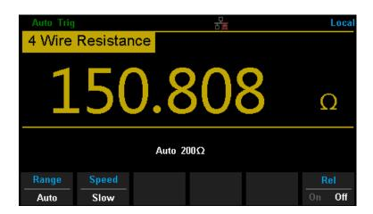
Diagram 2-15 4-Wire Resistance Measurement Interface
