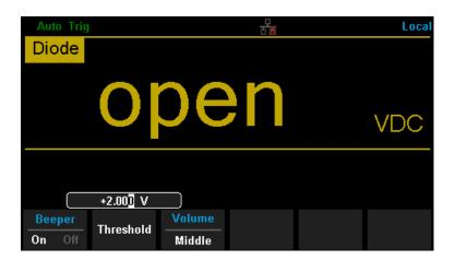
Diagram 2-25 Diode Test Interface
