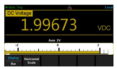
Diagram 2-63 Bar Meter Display Mode
