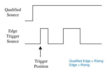
Click the *Qualified Setting* region to set the qualified source and threshold; Click the *Edge*Setting region to set the edge trigger source, threshold, and slope.
