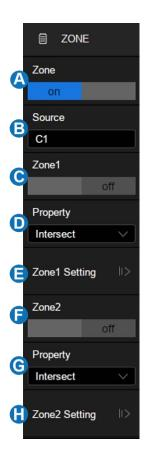
The zones can be created and moved by the mouse or by setting Zone > Zone Setting in the dialog box. The color of the zone's outline is consistent with the color of the specified source (Channel 1 = Yellow, etc...).
