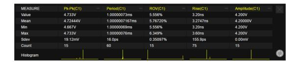
Click the histogram area of a parameter to enlarge it for details. You can move the large histogram window position around the display by dragging. Click the histogram of another parameter to switch to the corresponding enlarged histogram.
