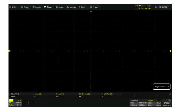
In Sequence mode, there is no waveform displayed on the screen until the acquisition is completed. During acquisition, there is a counter on the screen indicating the number of segments that have been acquired.
