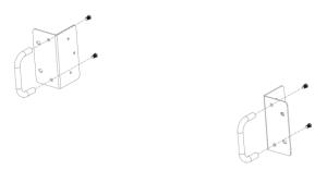
2. Install the rack flanges to the instrument using six M3×6 screws.
