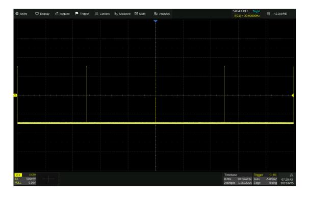
In normal mode, 5 pulses can be obtained on the screen with the sample rate of 1.25 GSa/s at the maximum memory depth.
