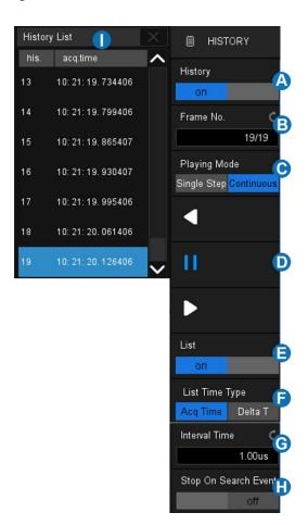
The oscilloscope automatically stores acquired frames. It can store up to 80,000 frames but the number may vary due to the memory depth and timebase settings. Turn on history mode, then the stored frames can be recalled and measured.
