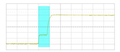
With a simple edge trigger, it is unlikely to trigger consistently on this anomaly. Thanks to the high waveform update rate of the SDS6000L, we can confirm there is bus contention happening by enabling the persistence display, as shown in the figure below:
