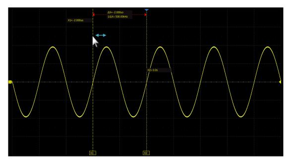
Click the display area of  $\triangle X$  (or  $\triangle Y$ ) in M1 mode and drag it to move the two cursors simultaneously, as shown in the figure below. This is equivalent to the operation on the cursor type X1-X2 or Y1-Y2.
