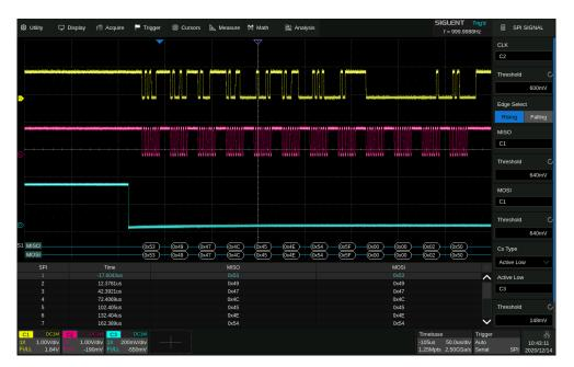
When the CS type is set to Clock Timeout, turn on Cursor, measure the clock idle time between frames as 150 us, and measure the interval between clock pulses as 1.28 us, then set the timeout to a value between 1.28 us and 150 us. In this example it is set to 5 us:
