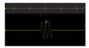
Adjust the horizontal position of the zoom area by dragging left and right in the zoom area of the main window or waveform in the Zoom window.
