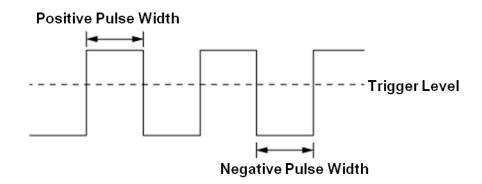
**Less than a time value** (≤) -- Trigger when the positive or negative pulse time of the input signal is lower than the specified time value. Below is an example of a trigger condition set to a positive pulse width < 100ns
