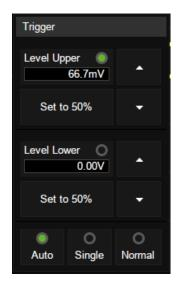
Click the *Level Upper* area in the quick menu to select the upper level, and then set the level value by the virtual keypad or the mouse wheel. To set the lower level is similar.
