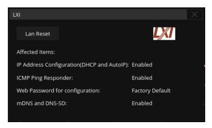
Click LAN Reset to restore the LAN defaults to your oscilloscope. It will enable automatic IP, ICMP Ping responder, and Multicast DNS, and reset the webserver password which is set in
