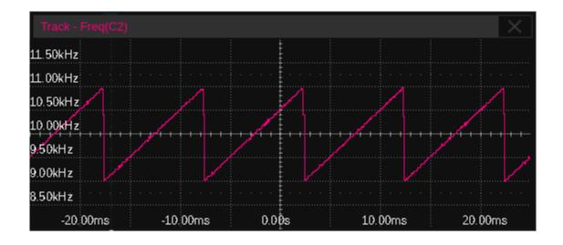
The upper limit of the statistic number in a frame is set in Statistics > AIM Limit, which means the values exceeding the limit will not be shown in the track plot. The upper limit is 1,000 by default and can be set to up to 65,000.
