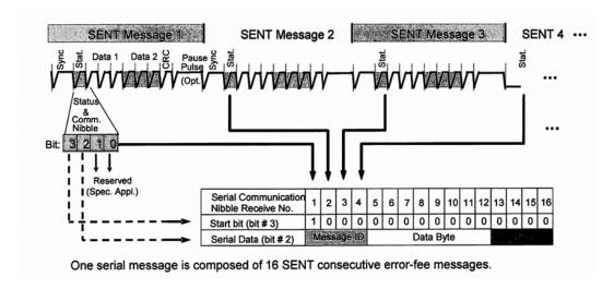
The serial message frame contains 21 bits of payload data. Two different configurations can be chosen and determined by the configuration bit (serial data bit #3, serial communication nibble No. 8):
