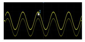
Click-and-drag the waveform up and down to move it on the vertical axis
