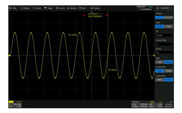
Fixed delay, timebase is changed to 100 ns/div, and the value of X cursors (-50 ns, 100 ns) remains fixed. The grid number of X cursors is changed to -0.5div, 1div.
