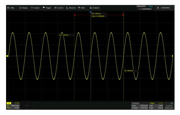
Fixed position, timebase is changed to 100 ns/div, and the grid number of X cursors (-1div, 2div) remains fixed. The value of X1 and X2 is changed to -100 ns, 200 ns.
