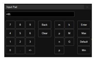
Let's use the operation of setting the "deskew" of a channel as an example: If the expected value is 65 ns, input "65" on the virtual keypad, and then choose n as the unit "ns" to complete the operation. On the virtual keypad, clicking the button n and n and n and n and n are the parameter to the maximum, minimum, and default values.
