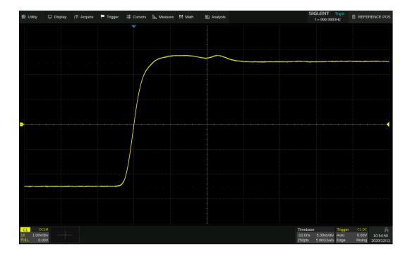
Fixed position, timebase is changed to 5 ns/div, the grid number of delay (-2div) remains fixed, while the horizontal delay changes to -10 ns
