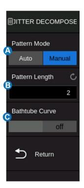
The result of jitter decomposition will be shown in the measured area. Users can add the jitter components interested, including measurement values, histogram, track, and spectrogram.
