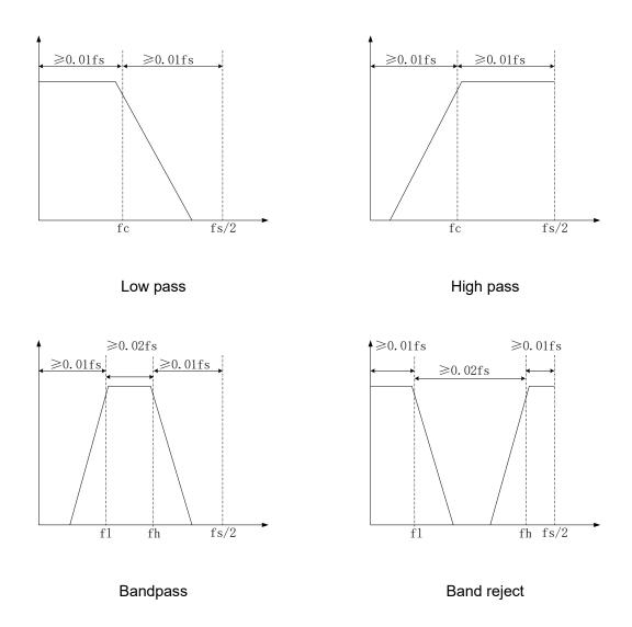
Take a Low pass filter as an example. It requires that the corner frequency (fc) is not less than 0.01\*fs (i.e. fc  $\geq 0.01*fs$ ), and the 0.01\*fs wide roll-off does not exceed the 1st Nyquist zone (i.e. (fs/2) - fc  $\geq 0.01fs$ ). If fs = 5 GSa/s, then the legal range of the corner frequency (fc) is 50 MHz~2450 MHz
