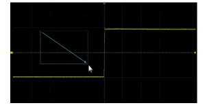
Click-and-drag along a diagonal line to create a zone or a histogram region. At the beginning of the drawing action keep the angle close to 45° so it can be recognized as the drawing box action
