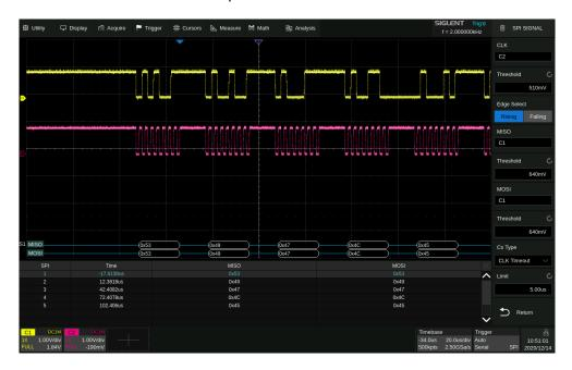
If the data width is set to be greater than 8 bits (such as 16 bits), measure the clock idle time between 8-bit data packets as 11.28 us, and then set the timeout time to a value between 11.28 and 150 us. In this example, it is set to 20 us:
