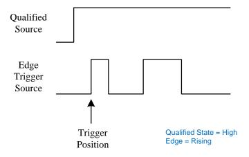
When the type is "Edge", the oscilloscope triggers at the first edge after the specified edge (Rising or Falling) of the qualified source; when the type is "Edge with Delay", a time limit condition is available.
