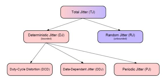
Figure 29.1 Jitter decomposition tree
