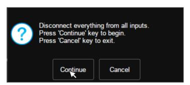
3. The oscilloscope will not respond to any operation until the self-cal is finished. After the self-cal is completed, click the screen to exit.
