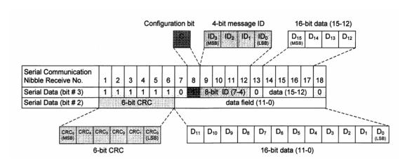
Frame (enhanced serial message with 8bits ID) —12-bit data and 8-bit message ID, the configuration bit is 0.
