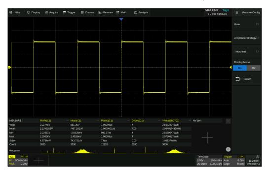
In M2 mode, up to 12 parameter measurements are displayed at a time. When statistics are enabled, they are distributed on the right side of the measurement item. Click a row to add or replace a measurement.
