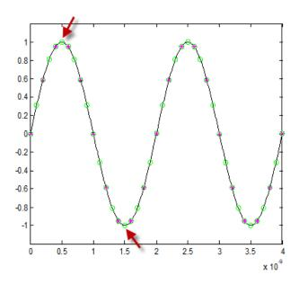
Error on vertical measurement after 2x interpolation
