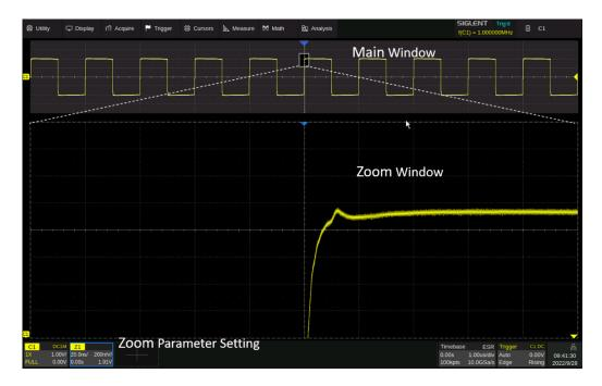
The area not covered by the gray background in the main waveform area is the range to be zoomed in (zoom area). Click the descriptor box of the zoom trace to recall the quick dialogs for setting the vertical and horizontal parameters of the zoom window.
