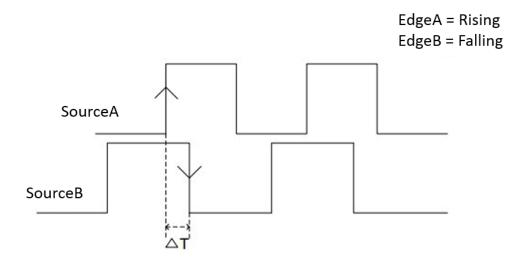
Click the SourceB Setting region to set the edge trigger source, threshold, and slope. Click the Limit Range and Upper / Lower Value region to set the delay time condition.
