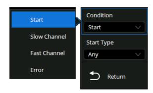
**Start** -- The oscilloscope will be triggered at the start of the message (after 56 synchronization ticks). You can select the type of message: Fast Channel Message, Slow Channel Message, or any.
