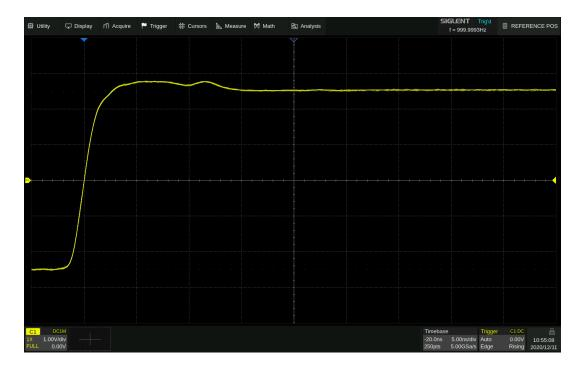
Fixed delay, timebase is changed to 5 ns/div, the horizontal delay value remains fixed, while the grid number of delay changes to -4div
