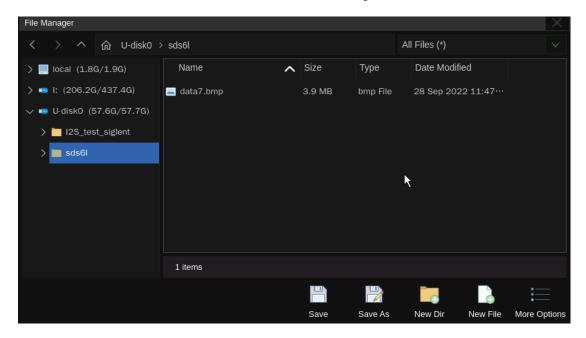
In step 4, if Save is selected instead of Save As , the system saves the file as the default file name SDS6xxxL\_BMP\_n.bmp, where n is an integer incrementing from 1. The default save path is \SIGLENT\.
