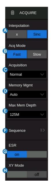
**Interpolation** -- At small timebase settings, the number of original points on the screen may be less than the number of display pixels in the grid area, so interpolation is necessary to display a continuous waveform. For example, at 1 ns/div timebase and 5 GSa/s sample rate, the number of original points is 50, but the grid area includes 1250 horizontal pixels. In this case, the oscilloscope needs to interpolate the original points by 25.
