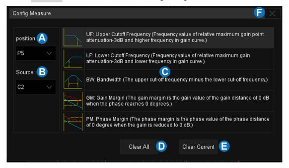
A. Set the position of measurement items, and support 5 measurement
