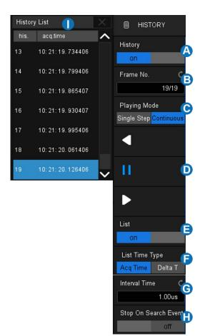
The oscilloscope automatically stores acquired frames. It can store up to 80,000 frames but the number may vary due to the memory depth and timebase settings. Turn on history mode, then the stored frames can be recalled and measured.
