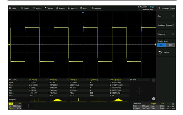
In M2 mode, up to 12 parameter measurements are displayed at a time. When statistics are enabled, they are distributed on the right side of the measurement item. Touch a row to add or replace a measurement.
