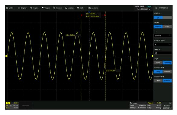
Fixed delay, timebase is changed to 100 ns/div, the value of X cursors (-50 ns, 100 ns) remains fixed. The grid number of X cursors is changed to -0.5div, 1div.
