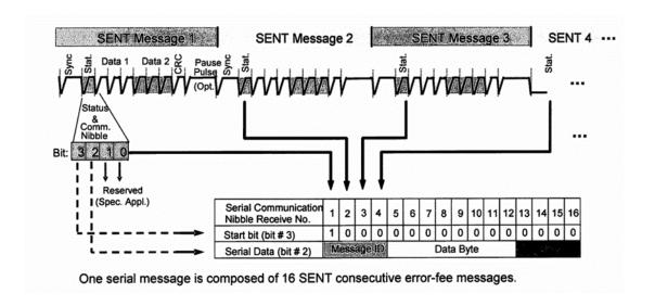
The serial message frame contains 21 bits of payload data. Two different configurations can be chosen determined by the configuration bit (serial data bit #3, serial communication nibble No. 8):
