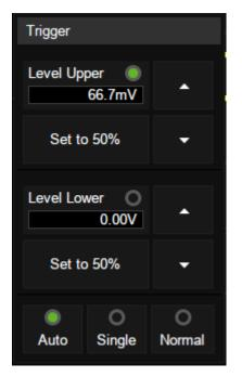
Touch the Level Upper area in the quick menu to select the upper level, and then set the level value by the virtual keypad or the Level knob on the front panel. To set the lower level is similar.
