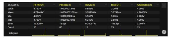
Touch the histogram area of a parameter to enlarge it for details. You can move the large histogram window position around the display by dragging. Touch the histogram of another parameter to switch to the corresponding enlarged histogram.
