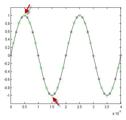
Error on vertical measurement after 2x interpolation
