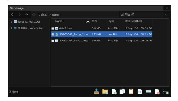
Fourth, touch the Recall icon and wait for the oscilloscope to finish recalling the setup.
