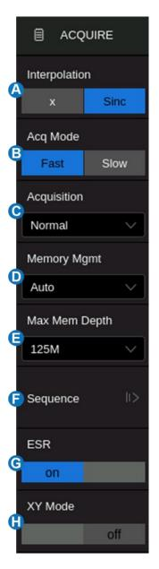
**Interpolation** -- At small timebase settings, the number of original points on the screen may be less than the number of display pixels in the grid area, so
