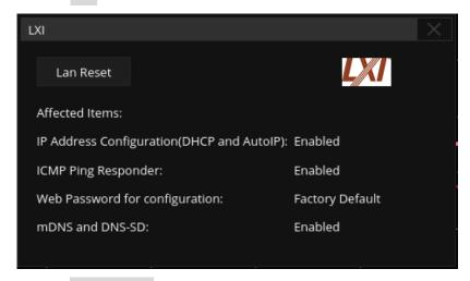
Touch *LAN Reset* to restore the LAN defaults to your oscilloscope. It will enable automatic IP, ICMP Ping responder, and Multicast DNS, and reset the webserver password which is set in **Utility**> I/O> Web Server.
