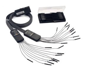
To connect the logic probe: Insert the probe, with the correct side facing up, until you hear a "click".
