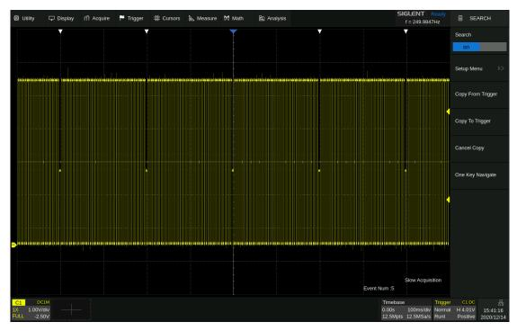
Turn on the Zoom function to observe the full view of the frame and the detail of the third dwarf pulse at the same time:
