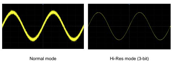
Hi-Res acquisition does not require the signal to be periodic, nor does it require stable triggering, but due to the digital filtering, the system bandwidth of the oscilloscope will degrade in Hi-Res mode. The higher the enhanced bits, the lower the bandwidth. The following table shows the relationship between Hi-Res bits and bandwidth:
