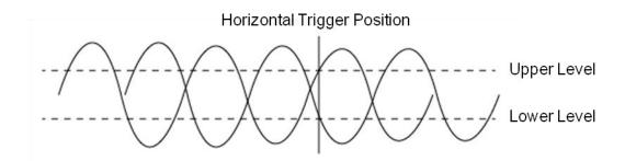
If the lower and the upper trigger levels are both within the waveform amplitude range, the oscilloscope will trigger on both rising and falling
