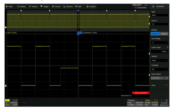
Press the Run/Stop button on the front panel to stop the acquisition, and then follow the steps Navigate Type to select "Search Event". The following figure shows the first dwarf pulse. In this example, the list is enabled and the time labels of each event are shown in the list.
