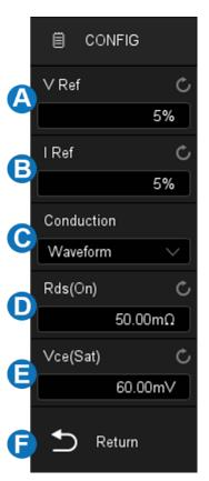
**Rds (on)** -- In the on area (where the voltage level is lower than the voltage reference (adjustable)), the power calculation formula is  $P = I^2 * Rds$  (on). In the off area (where the current level is lower than the current reference (adjustable)), the power calculation formula is P = 0 watt.
