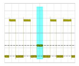
First, set the trigger type to Runt to trigger on the dwarf pulse. See the section "Runt Trigger" for details.
