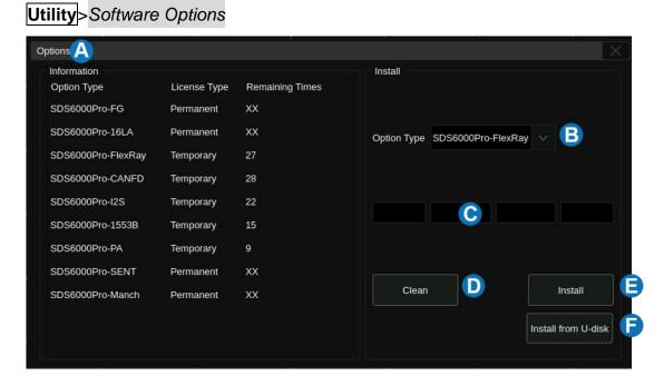
A. Option information display area. When the option is not activated, the license type is displayed as "Temporary" and can be tried up to 30 times.
