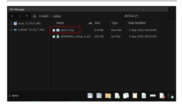
In step 4, if Save is selected instead of Save As, the system saves the file as the default file name SDS6xx4A\_BMP\_n.bmp, where n is an integer incrementing from 1. The default save path is \SIGLENT\.
