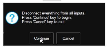
3. The oscilloscope will not respond to any operation until the self-cal is finished. After the self-cal is completed, touch the screen or press any button to exit.
