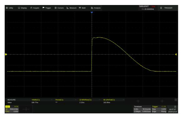
In the example, 53969 pulses can be obtained with the sample rate of 5 GSa/s at the maximum memory depth.
