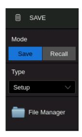
Third, select the "\Udisk0\sds6a\" directory in the file manager, and then select the setup file "SDS6054A\_Setup\_1.xml"
