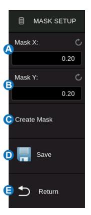
Set the values for *Mask X* and *Mask Y* (in divisions of display graticule), and then perform *Create Mask* to generate the mask. The horizontal and vertical adjustment range is 0.08~4.00 div.
