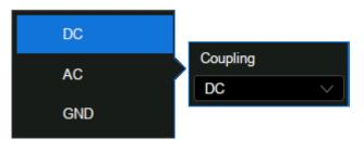
List: Sets parameters with more than two options, such as coupling mode of channels. Touch the parameter region, and then select the expected option from the pop-up list.
