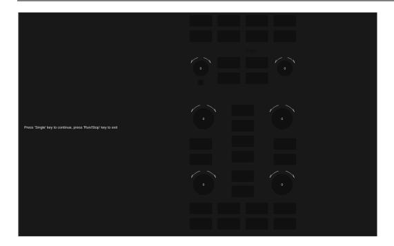
Press the "Single" button and the first LED on the front panel will light. The corresponding position of the key on the screen will also change color. Press the "Single" button to check the next button. Press the "Single" button consecutively until all the backlights are tested. Press the "Run/Stop" button to exit the LED test.
