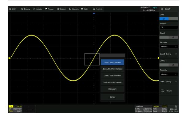
Once a zone is created, it can be moved by dragging. Just touch and hold the zone box and use a dragging gesture.
