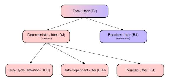
Figure 31.1 Jitter decomposition tree
