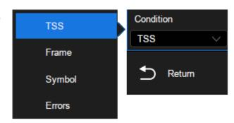
• **TSS**— The oscilloscope triggers on the transmission start sequence.
