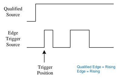
Touch the *Qualified Setting* region to set the qualified source and threshold; Touch the *Edge Setting* region to set the edge trigger source, threshold, and slope.
