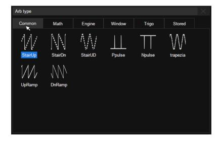
There are 6 tabs in the window. Under each tab, a catalog of waveforms is listed.
