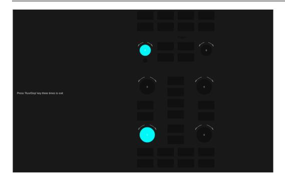
**Knob test:** Turn each knob clockwise, counter-clockwise, and press down. Observe whether the value on the corresponding knob (default 0) on the screen increases or decreases in real-time and whether the knob lights up when it is pressed.
