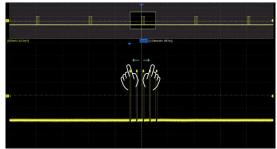
Adjust the horizontal scale of Zoom window by horizontal pinch and spread in the zoom area of the main window or the Zoom window.
