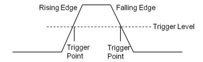
Touch the *Source* area to select trigger source, and touch the *Slope* area to select rising, falling, or alternating.
