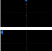
Trigger Delay Indicator locates where the waveform triggers on the horizontal axis...
