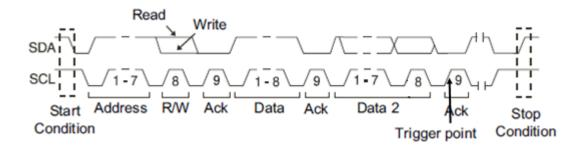
**10 Address & Data** — If all bits match, then trigger on the Ack bit followed by the Data.
