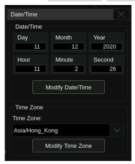
Touch the text box of Hour, Minute, Second, Day, Month, and Year to edit these fields. Touch the *Modify Date/Time* button to perform the change. Touch the text box of Time Zone to select the time zone. Touch the *Modify Time Zone* button to perform the change.
