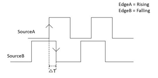
Touch the *SourceB Setting* region to set the edge trigger source, threshold, and slope. Touch the *Limit Range* and *Upper/Lower Value* region to set the delay time condition.
