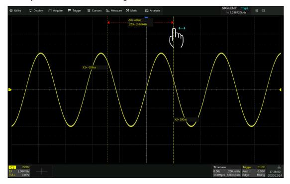
Touch the display area of  $\triangle X$  (or  $\triangle Y$ ) in M1 mode and drag it to move the two cursors simultaneously, as shown in the figure below. This is equivalent to the operation on the cursor type X1-X2 or Y1-Y2.
