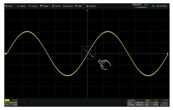
When the finger moves out of the screen, a menu pops up for selecting the zone and setting the zone properties:
