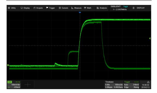
In this case zone trigger is a quick and simple way to capture the waveform. Enable the zone trigger, and draw a box to intersect with the bus contention part, as shown in the figure below:
