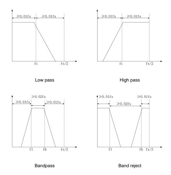
Take a Low pass filter as an example. It requires that the corner frequency (fc) is not less than 0.01\*fs (i.e.  $fc \ge 0.01*fs$ ), and the 0.01\*fs wide roll-off does not exceed the 1\*f Nyquist zone (i.e.  $(fs/2)-fc \ge 0.01fs$ ). If fs = 5 GSa/s, then the legal range of the corner frequency (fc) is 50 MHz~2450 MHz.
