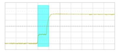
With a simple edge trigger, it is unlikely to trigger consistently on this anomaly. Thanks to the high waveform update rate of the SDS6000A, we can confirm there is bus contention happening by enabling the persistence display, as shown in the figure below:
