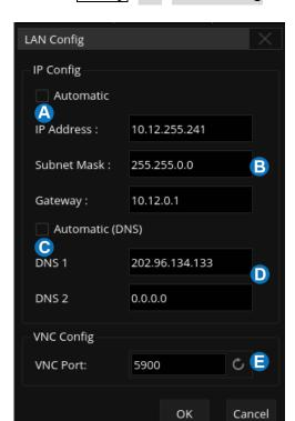
Perform Utility > I/O > LAN Config to open the LAN Config dialog box.
