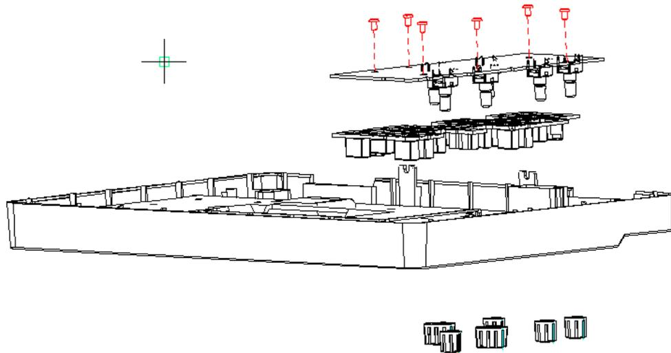
Figure 17 To remove the rubber keypad and keyboard
