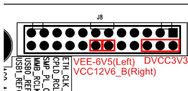
Figure 26 Test points for the LCD power supplies
