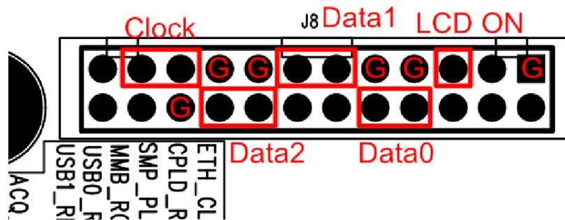
Figure 27 Test points for LCD signal
