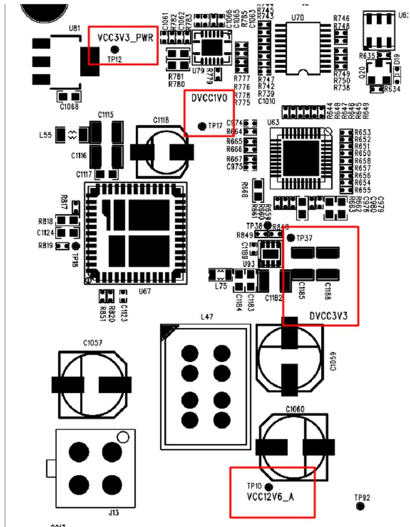
Figure 19 Test points for the Acquisition board power supplies
