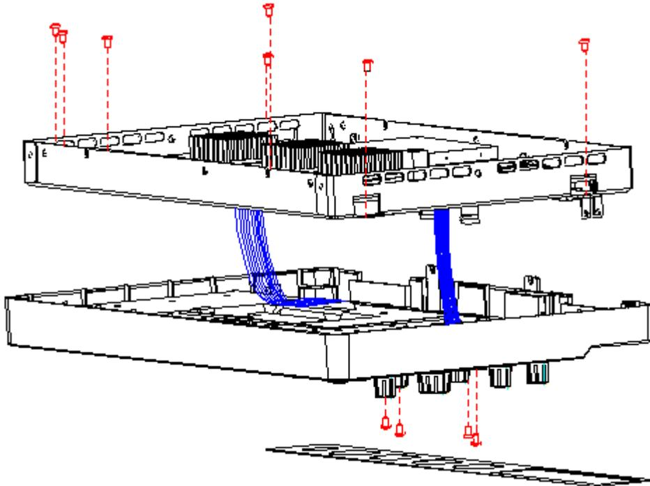
Figure 16 To remove the mainboard and front panel
