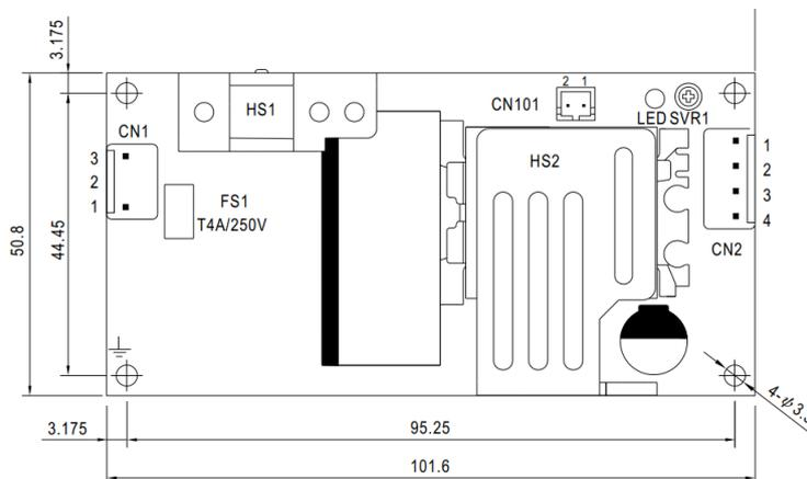
Figure 18 Power supply module mechanical drawing
