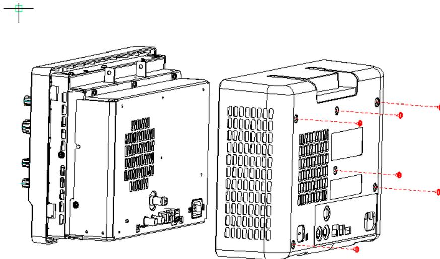
Figure 12 To remove the rear cover
