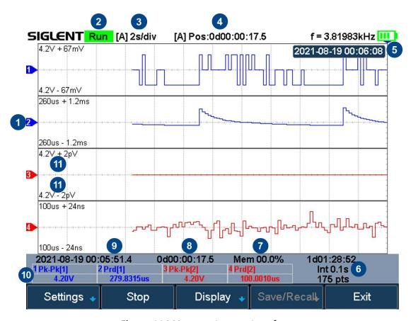
Figure 116 Measure Logger Interface
