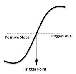
You can adjust the trigger level for a selected analog channel by pressing the **Trigger Level** button and turning the **Universal Knob**.
