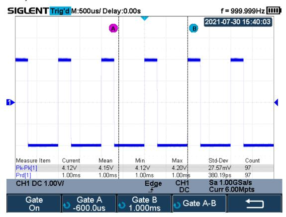
Figure 85 Gate Measurement
