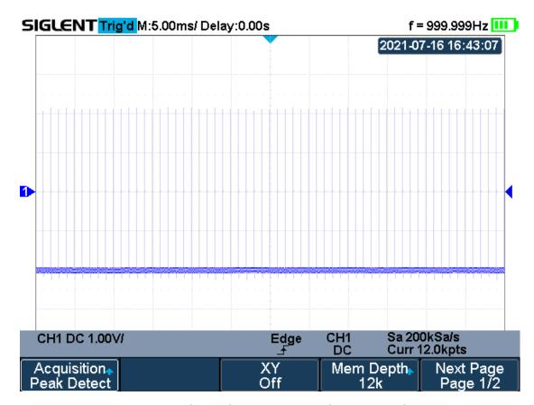
Figure 20 Pulse With 0.1% Duty, Peak Detect Mode
