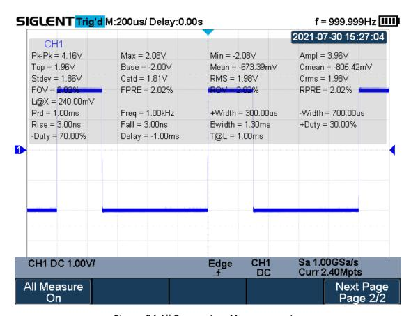
Figure 84 All Parameters Measurement
