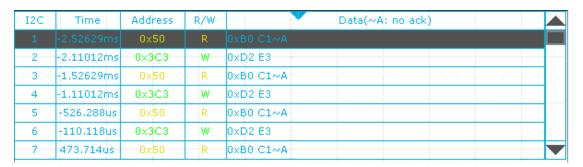
Figure 42 I2C Decode List Display
