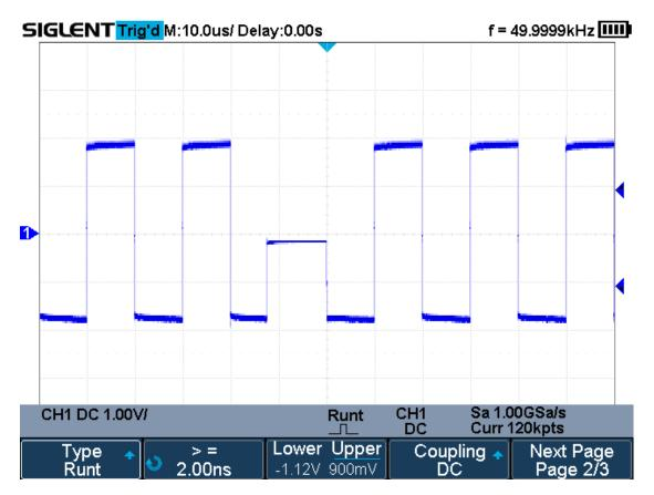
Figure 36 Runt Trigger
