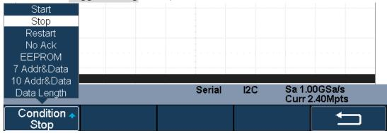
Figure 40 I2C TRIGGER Menu
