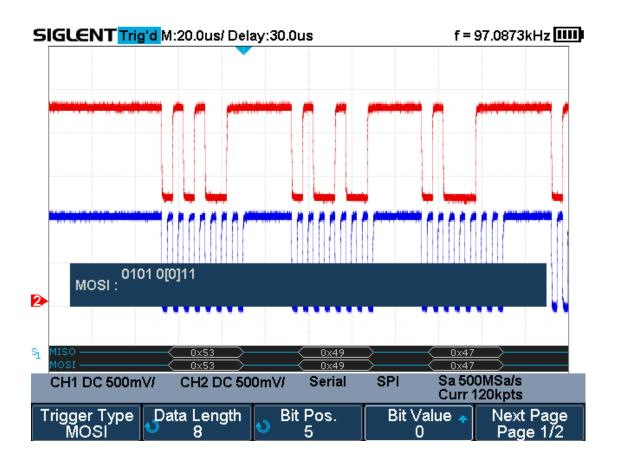
If the data width is set to be greater than 8 bits (such as 16 bits), the clock idle time between 8-bit data packets T2, and then set the timeout time to a value between T1/2+T2 and T3.
