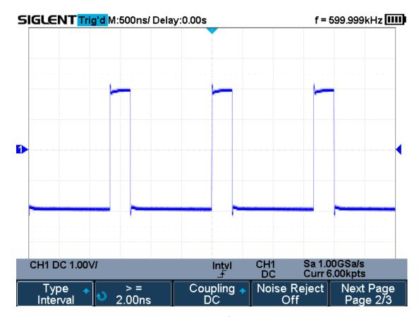
Figure 33 Interval Trigger
