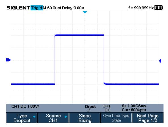
Figure 35 State Dropout Trigger
