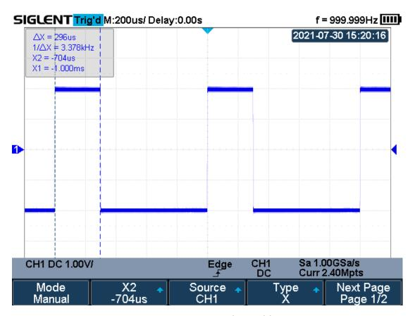
Figure 77 Measure Pulse Width
