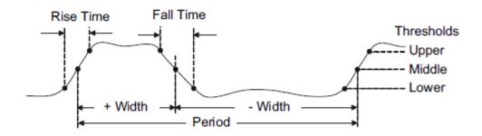
Figure 81 Time Measurements
