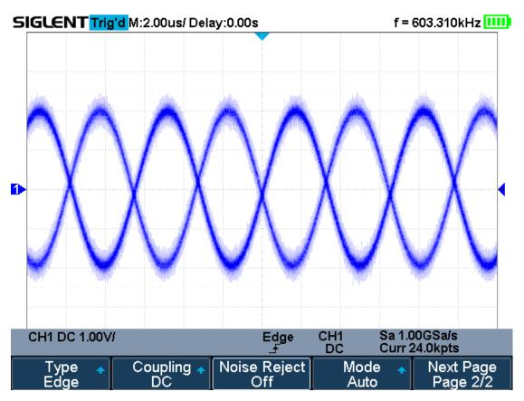
Figure 25 Turn off the Noise Reject
