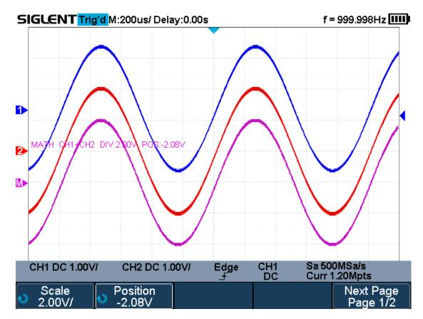
Figure 62 C1+C2 Waveform
