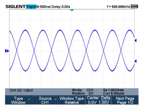
Figure 32 Relative Window Trigger
