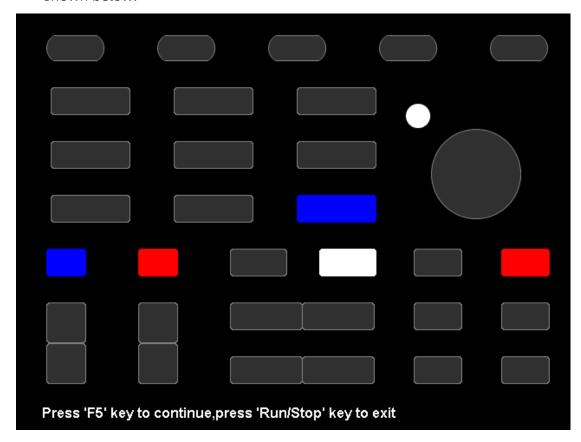
Figure 98 LED Test
