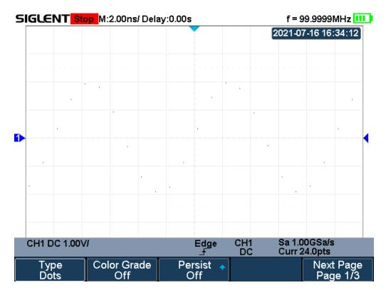
Figure 15 Display Type Set to Dots
