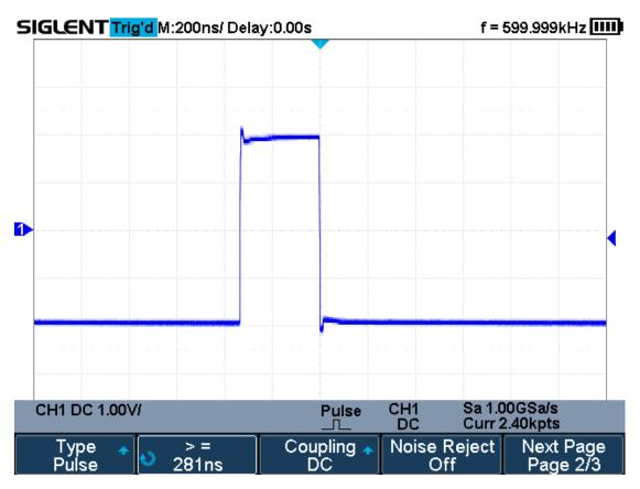
Figure 29 Pulse Trigger
