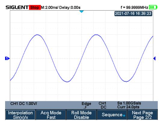
Figure 17 Sinx/x Interpolation
