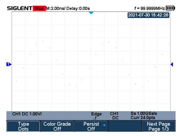
Figure 87 Dots Display
