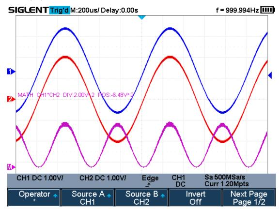
Figure 63 C1\*C2 Waveform
