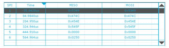
Figure 49 SPI Decode List Display
