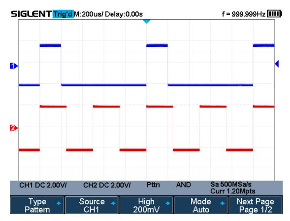
Figure 37 Pattern Trigger
