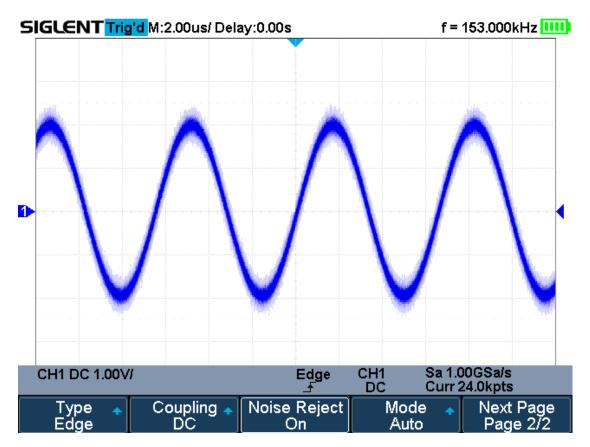
Figure 26 Turn on the Noise Reject
