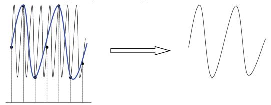
Waveform Leakage: when the sample rate is too low, the waveform reconstructed from the sample data cannot reflect all the actual signal information.
