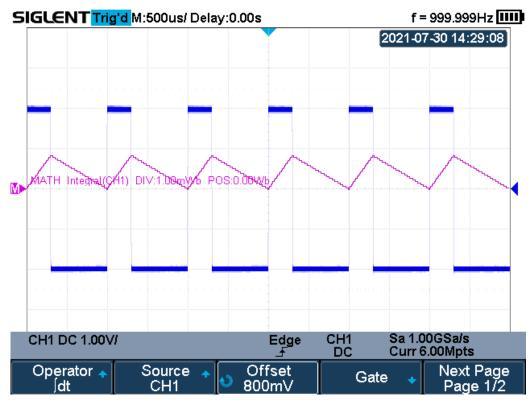
Figure 75 Integral with Offset
