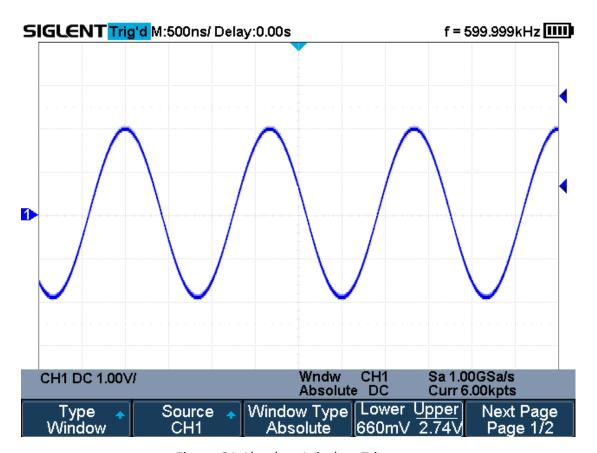
Figure 31 Absolute Window Trigger
