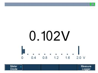
Figure 108 Diode Measurement
