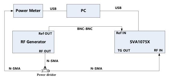
Figure 3-1 Absolute amplitude accuracy connections
