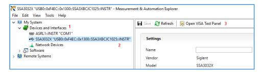
4. Click the "Open VISA Test Panel" option button, and then the following Interface will appear. Then click the "Input/Output" option button and click the "Query" option button to view the Read operation information.
