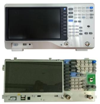
Figure 4-2 Removing the front panel
