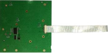
Figure 4-5 Removing the LCD and keyboard
