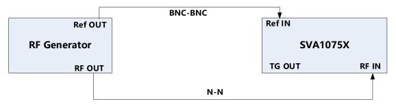
Figure 3-4 Phase noise verification connections
