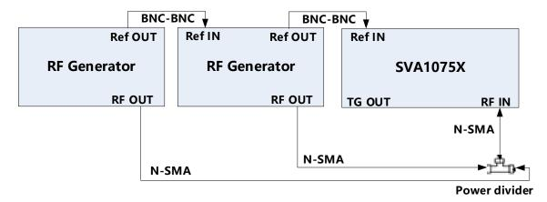
Figure 3-5 TOI verification connections
