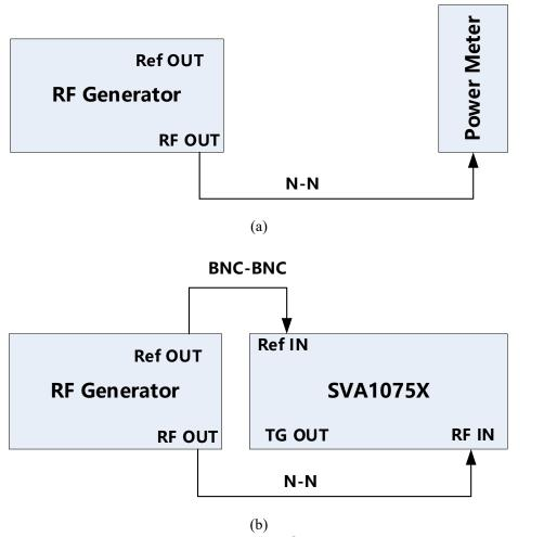
Figure 3-9 connecting test instruments for Input Attenuation Error Test
