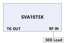
Figure 3-3 DANL verification connections
