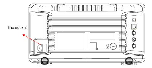
Figure 1-1 Connect the power cord
