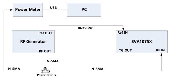
Figure 3-2 Frequency response connections
