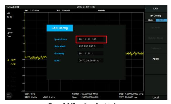
Figure 2-2 IP configuration interface
