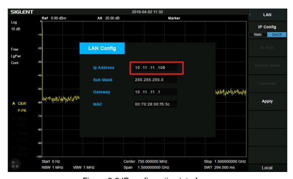
Figure 2-2 IP configuration interface
