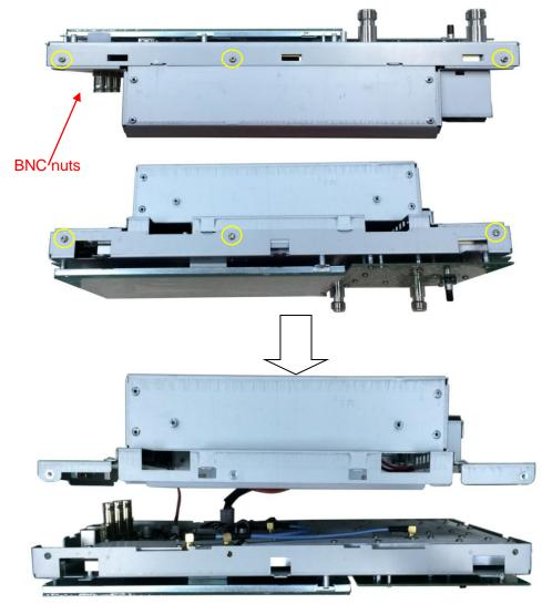
Figure 4-3 Removing the rear metal cover
