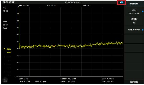
Figure 2-1 USB drive has been properly recognized
