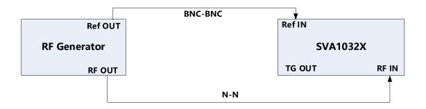
Figure 3-4 Phase noise verification connections
