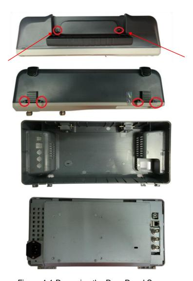
Figure 4-1 Removing the Rear Panel Screws
