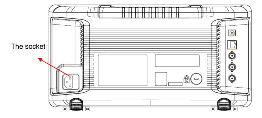
Figure 1-1 Connect the power cord
