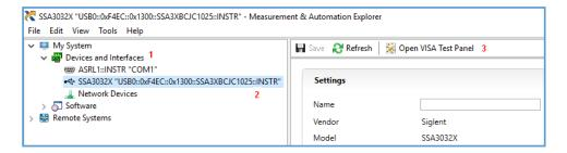
4. Click the "Open VISA Test Panel" option button, and then the following The interface will appear. Then click the "Input/Output" option button and click the "Query" option button to view the Read operation information.
