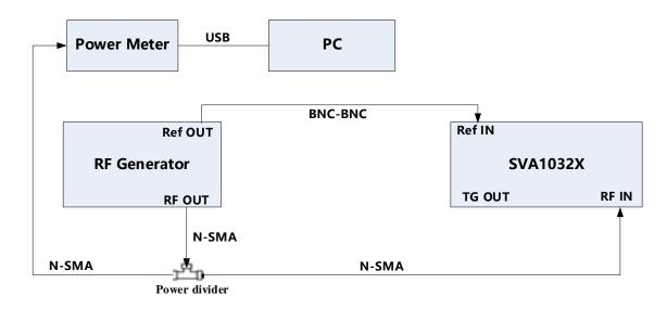
Figure 3-2 Frequency response connections
