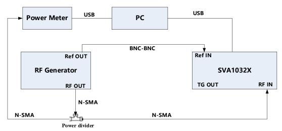
Figure 3-1 Absolute amplitude accuracy connections
