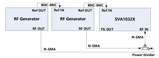
Figure 3-5 TOI verification connections
