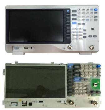
Figure 4-2 Removing the front panel
