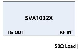
Figure 3-3 DANL verification connections
