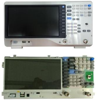
Figure 4-2 Removing the front panel
