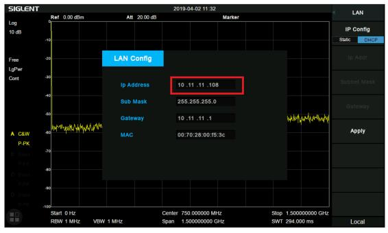
Figure 2-2 IP configuration interface
