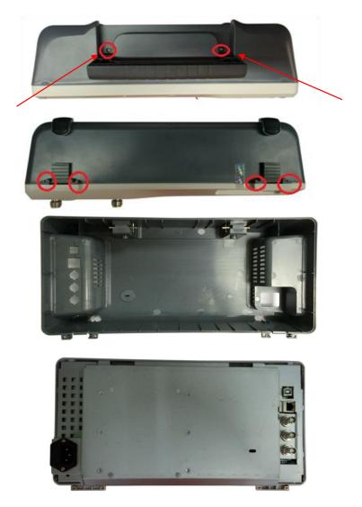
Figure 4-1 Removing the Rear Panel Screws
