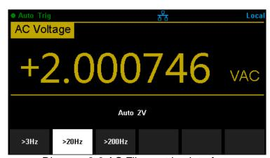
Diagram 2-6 AC Filter setting interface
