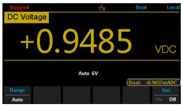
Diagram 2-24 Dual-display function Interface (Main DCV, Vice DCI)
