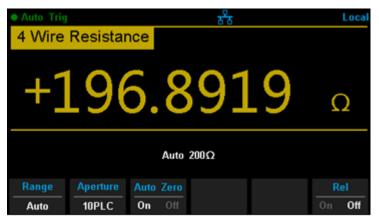
Diagram 2-14 4 Wire Resistance Measurement Interface
