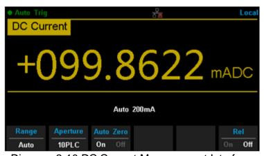
Diagram 2-10 DC Current Measurement Interface
