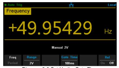
Diagram 2-8 Set Up the Gate Time
