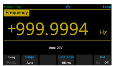
Diagram 2-16 Fequency Measurement Interface
