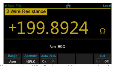
Diagram 2-13 2 Wire Resistance Measurement Interface
