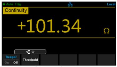
Diagram 2-7 Set Up the Short-circuit Resistance
