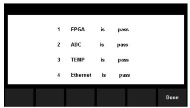
Diagram 2-39 Chip Test Interface
