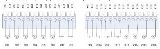
Notes: [1] Each channel of CH1-CH12 can be used for switching measurement of voltage, 2-W resistance, capacitance, frequency, continuity, diode, temperature, etc. CH13-CH16 channels are fixed for current measurement below 2.2A.
