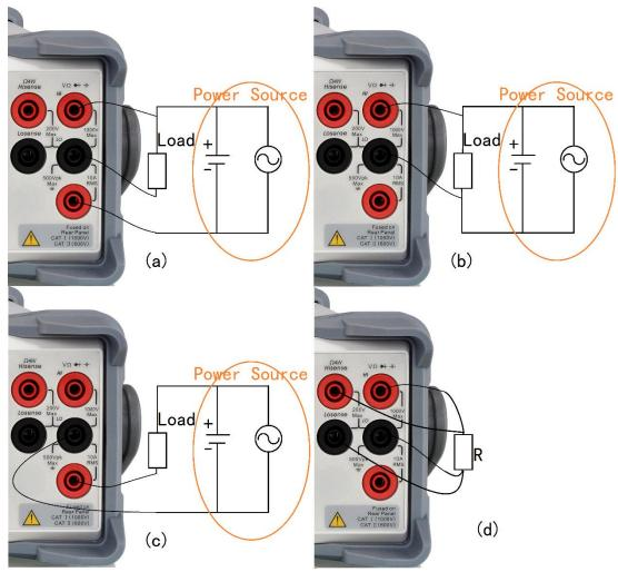
Diagram 2-25 Dual-display wiring example
