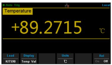
Diagram 2-20 Temperature Measurement Interface
