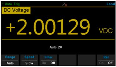
Diagram 2-9 DC Voltage Measurement Interface
