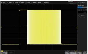
Segmented memory collection will store the waveform into multiple memory segments (up to 80,000) and each segment will store a triggered waveform as well as the dead time information. The interval between segments can be as small as  $1.3\mu s$ . All of the segments can be played back using the History function
