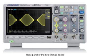
• 7 -inch TFT -LCD display with 800 \* 480 resolution
