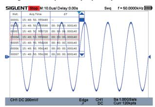
Playback the latest triggered events using the history function. Segmented memory collection will store trigger events into multiple (Up to 80,000) memory segments, each segment will store triggered waveforms and timestamps for each frame.
