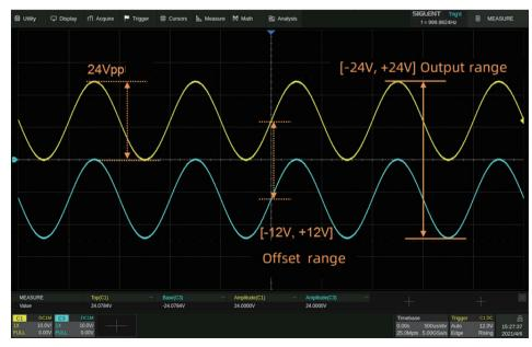
24Vpp analog output superimposed with  $\pm$  12 Vdc offset, providing a maximum output range of  $\pm$  24 V (48 V).
