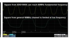
Benefitting from a special square-wave generating circuitry, the Square from the SDG1000X breaks the 60 MHz bandwidth barrier, reaching rise/fall times of less than 4.2 ns, and frequencies up to 60 MHz.
