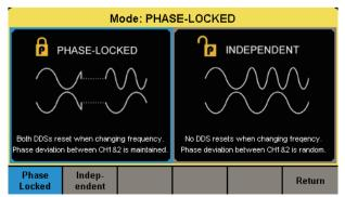
"Phase-Locked" mode automatically aligns the phases of each output. While "Independent" mode permit the two channels to be used as two independent generators. Independent mode also smoothes parameter (frequency, amplitude) changes made to an active channel.
