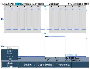
The SHS800X/SHS1000X series can search events specified by the user in a frame. It can also navigate by time (delay position) and historical frames.
