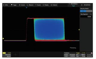
Segmented memory collection will store the waveform into multiple memory segments (up to 100,000) and each segment will store a triggered waveform as well the dead time information. The dead time between segments can be as small as 2  $\mu s$ . All of the segments can be played back using the History function
