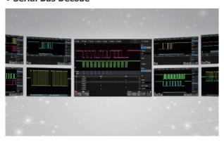
Display the decoded characters through the events list. Bus protocol information can be quickly and intuitively displayed in tabular form. I2C, SPI, UART, CAN, LIN, CAN FD, FlexRay, I2S, MIL-STD-1553B, SENT, and Manchester are supported
