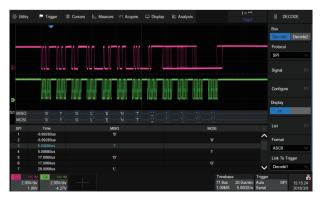
Display the decoded characters through the events list. Bus protocol information can be quickly and intuitively displayed in tabular form. I2C, SPI, UART, CAN, LIN, CAN FD, FlexRay and I2S and MIL-STD-1553B are supported
