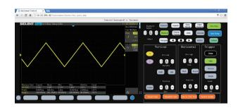
With the new embedded web server, users can control the SDS2000X-E from a simple web page. This provides wonderful remote troubleshooting and monitoring capabilities. The web page has PC and mobile styles that include an embedded virtual control panel.
