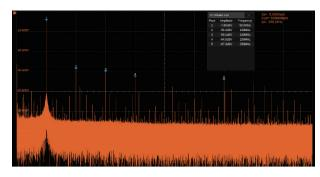
Hardware-accelerated FFT supports up to 8 Mpts operation. This provides high-frequency resolution with a fast refresh rate. The FFT function also supports a variety of window functions so that it can adapt to different spectrum measurement needs. Three modes (Normal, Average, and Max hold) can satisfy different requirements for observing the power spectrum. Auto peak detection and markers are supported.
