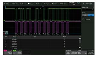
In addition to the decoder lanes correlated to the waveform, bus protocol information can be displayed in tabular form. I2C, SPI, UART, CAN, LIN, CAN FD, FlexRay, I2S and MIL-STD-1553B are supported.
