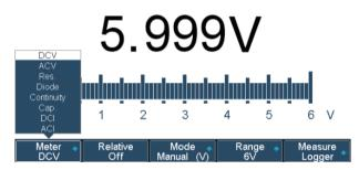
6000 count digital multimeter featured function of DCV, true RMS ACV, DCI, ACI, Diode, Resistance, Capacitance, and Continuity.
