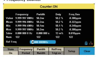
8-digit hardware frequency counter with statistics function and input range of 0.1 Hz  $\sim$  400 MHz.
