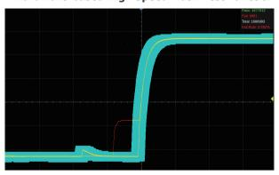
The oscilloscope utilizes a hardware-based Mask Test function, performing up to 18,000 Pass / Fail decisions each second. It is easy to generate user-defined test templates to provide trace mask comparisons, making it suitable for long-term signal monitoring or automated production line testing
