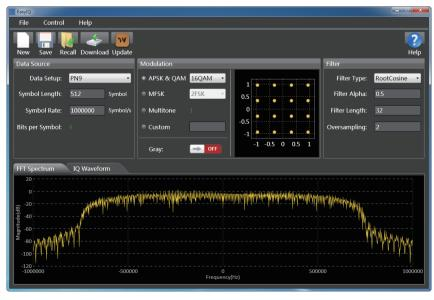
IQ waveforms can be generated by the PC software EasyIQ.
