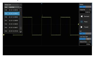
History function can record up to 80,000 frames of waveforms. The recording is executed automatically so that the customer can playback the history waveforms at any time to observe unusual events and quickly locate the area of interest using the cursors or measurements. The failed frames of the Mask Test can be stored as history
