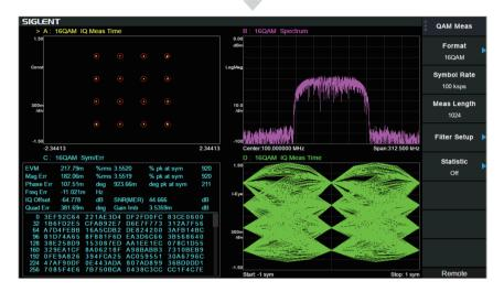
The SDG6000X supports popular modulation types such as ASK, FSK, PSK, and QAM. Proprietary resampling technology provides excellent EVM performance at arbitrary symbol rates between 250 Symb/s ~ 37.5 MSymb/s. Built-in digital quadrature modulator provides the possibility to generate IQ signals from baseband to 500 MHz intermediate frequency.
