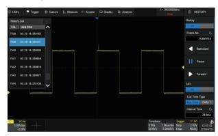
History function can record up to 100,000 frames of waveforms. The recording is executed automatically, so that the customer can play back the history waveforms at any time in order to observe unusual events and quickly locate the area of interest using the cursors or measurements
