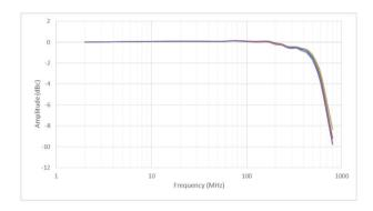
500 MHz bandwidth (at 2 GSa/s sample rate with 500 MHz bandwidth option).
