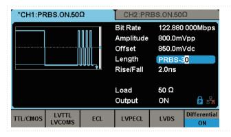
Preset common logic levels such as TTL, LVCMOS, LVPECL and LVDS. An added differential mode provides an easy way to generate differential signals using the both channels.
