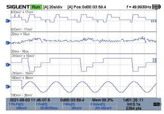
The measurement Logger is the mode of logging the measurement value for a long time. For the amount of measurement data is relatively small, to process quickly, the data is logged in memory. After stopping logging, the data can be saved into the internal flash or external U disk.
