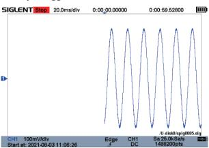
The Sample Logger is the mode of logging the sampling points for a long time. For there are many sampling points to log, they are logged into the internal flash or external U disk in real-time. After stopping logging, the user can recall the sampling points on the oscilloscope, or analyze the saved data on the computer.
