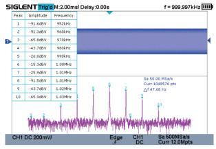
The new math co-processor enables FFT analysis of incoming signals using up to 1 M samples per waveform. This provides high-frequency resolution with a fast refresh rate. The FFT function also supports a variety of window functions so that it can adapt to different spectrum measurement needs. Support Peaks, Markers, a variety of numbers.
