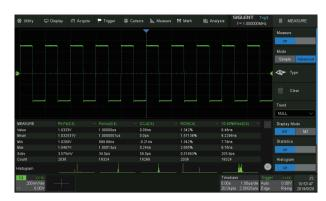
Parameter measurements includes 4 categories: Vertical, Horizontal, Miscellaneous and Channel Delay providing a total of 50+ different types of measurements. Measurements can be performed within a specified gate period. Measurements on Math, Reference and History frames are
