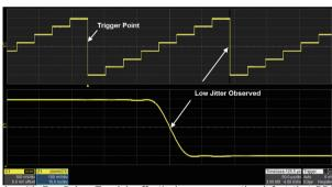
As with EasyPulse, TrueArb effectively overcomes the defect that DDS may cause the one-clock-jitter in arbitrary waveforms.
