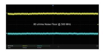
Low noise floor: Only 80  $\mu V$  rms at 500 MHz bandwidth.
