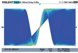
The color temperature display is similar to the intensity-graded trace function, but the trace occurrence is represented by different colors (color "temperature") as opposed to changes in the intensity of one color. Red colors represent events that occur more frequently, while blue is used to mark points that occur less frequently.
