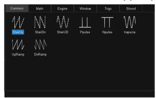
The built-in waveform generator can output waveforms with up to 25 MHz frequency and  $\pm 3$  V amplitude. Six basic waveforms together with multiple types of predefined waveforms and as user-defined arbitrary waveforms are supported
