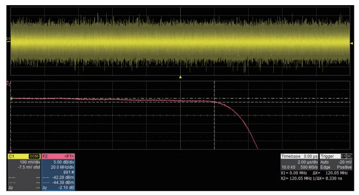
The bandwidth of analog channels proves to be greater than 120 MHz, via doing a frequency response test with white noise.
