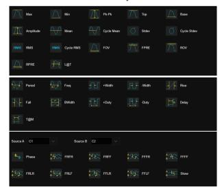
Parameter measurements includes 3 categories: horizontal, vertical and CH delay providing more than 70 different types of measurements. Measurements can be performed within a specified gate period. Measurements on Math, Reference and History frames are supported
