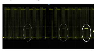
With a waveform update rate of up to 170,000 wfm/s, the oscilloscope can easily capture unusual or low-probability events. In Sequence mode, the waveform capture rate can reach 750,000 wfm/s
