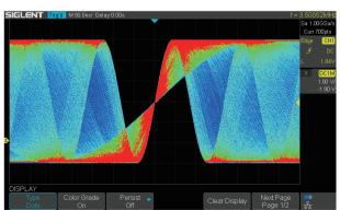
The color temperature display is similar to the intensity-graded trace function, but the trace occurrence is represented by different colors (color "temperature") as opposed to changes in the intensity of one color. Red colors represents the more frequent events, while blue is used to mark points that occur less frequently.
