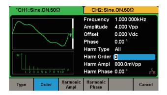
Up to 10 harmonics may be generated. Amplitude and phase of each harmonic can be set independently.
