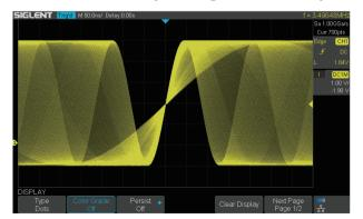
SPO display technology provides for fast refresh rates. The resulting intensity-graded trace is brighter for events that occur with more frequency and dims when the events occur with less frequency.
