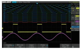
16 digital channels enables users to acquire and trigger on digital input channels and view both digital and analog waveforms simultaneously with one instrument.
