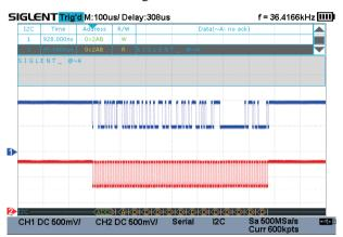
SHS800X/SHS1000X displays the decoding through the events list. Bus protocol information can be quickly and intuitively displayed in a tabular format.
