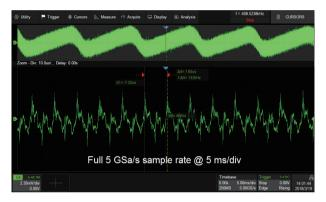
Using hardware-based Zoom technique and record length of up to 250 Mpts, users are able to select a slower timebase without compromising the sampling rate, and then quickly zoom in to focus on the area of interest
