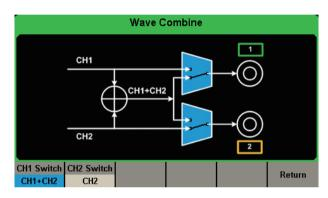
Capable of combining the waveforms of 2 channels from internal, providing more flexible tools to generate complex waveforms.
