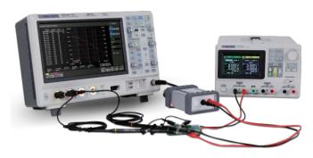
The SDS2000X Plus can control the built-in waveform generator or any stand-alone SIGLENT SDG device to scan the amplitude and phase response over frequency of passive or active circuits. The data is presented as Bode Plot. This makes it possible to replace expensive network analyzers in less demanding applications.
