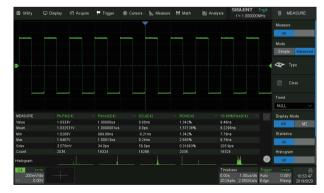
Statistics show the current value, maximum value, minimum value, standard deviation, and mean value of up to 12 parameters simultaneously. A histogram is available to show the probability distribution of a parameter. Trend and Track are available to show the parameter value vs. time.
