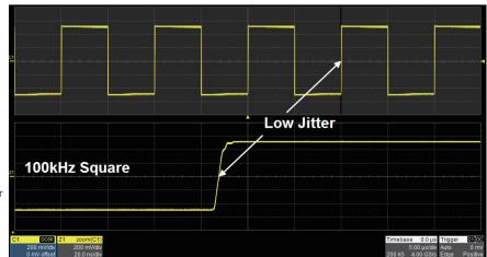
The Square wave exhibits the same excellent jitter performance as the Pulse waveform.
