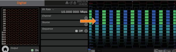
Purchase the corresponding digital bus kit to get 16-channel LVTTL or LVDS output with a bit rate of 1  $\mu$ bps  $\sim 1$  Gbps. Combine the digital bus with the analog channels to realize mixed-signal outputs.
