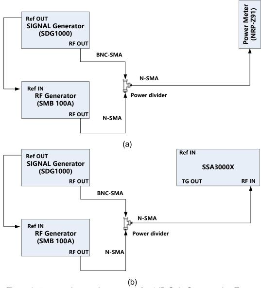
Figure 3-7 connecting test instruments for 1dB Gain Compression Test
