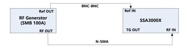
Figure 3-4 Phase noise verification connections
