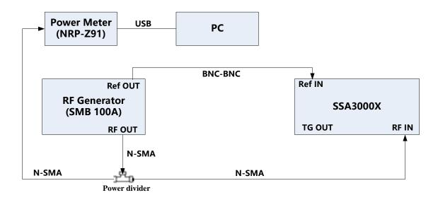
Figure 3-2 Frequency response connections
