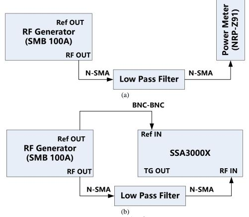
Figure 3-8 connecting test instruments for Second Harmonic Distortion Test
