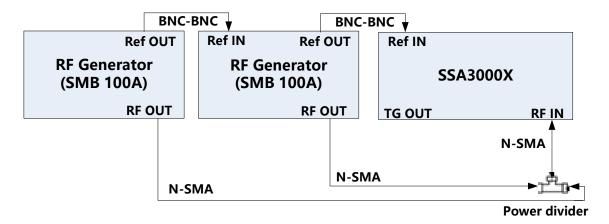
Figure 3-5 TOI verification connections
