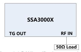
Figure 3-3 DANL verification connections
