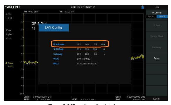
Figure 2-2 IP configuration interface
