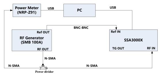
Figure 3-1 Absolute amplitude accuracy connections
