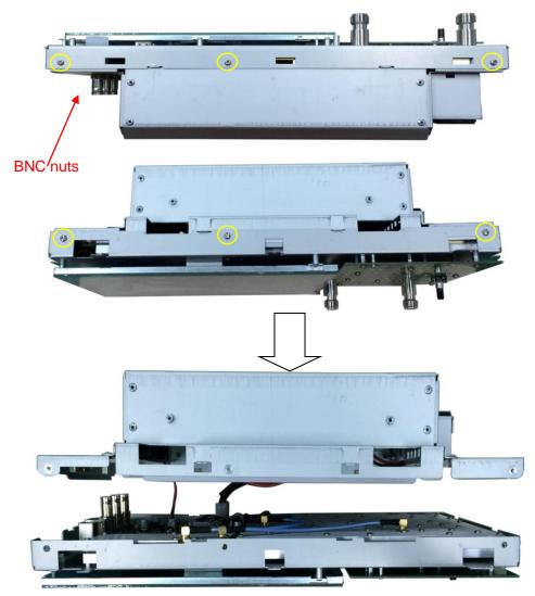
Figure 4-3 Removing the rear metal cover
