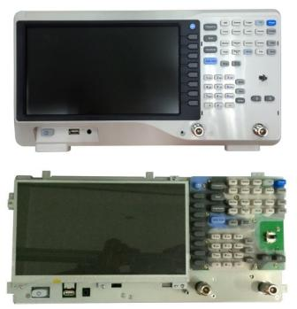
Figure 4-2 Removing the front panel
