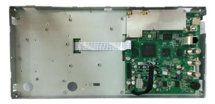
Figure 4-4 View of front panel subassembly with main board (upper) and with main board removed (lower)
