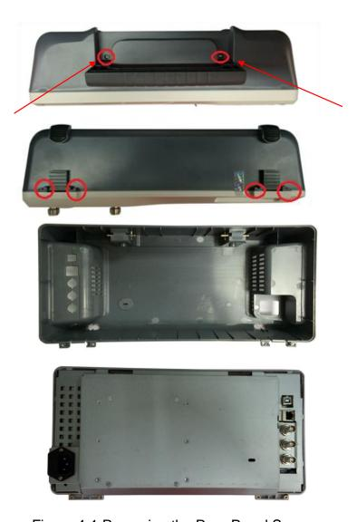
Figure 4-1 Removing the Rear Panel Screws
