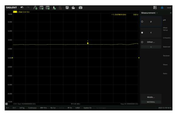
Figure 15-15 Permittivity Measurement Results (PEI Material)
