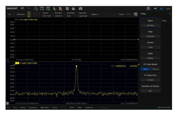
Figure 11-4 [Freq] key to set SA frequency parameters
