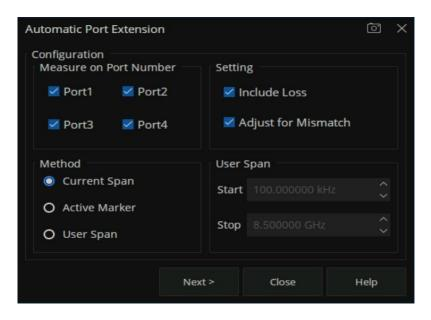
Figure 7-6 Automatic port extension setting interface
