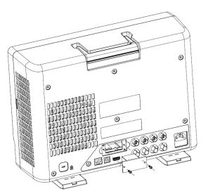
Figure 5-9 OCXO option installation guide
