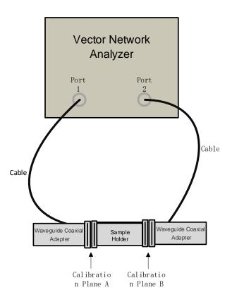
Figure 15-14 Schematic Diagram of Equipment Connection
