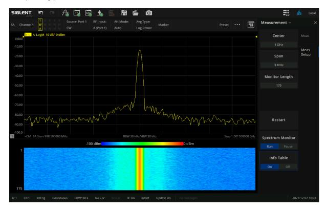
Figure 11-18 Spectrum Monitor
