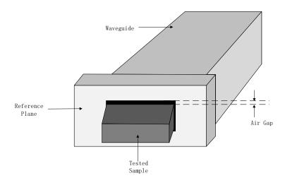
Figure 15-13 Schematic Diagram of Sample Installation
