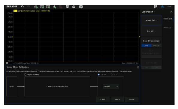
Characterization calibration mixer/filter combination configuration interface
