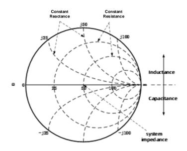
Figure 6-6 Schematic diagram of Smith circle
