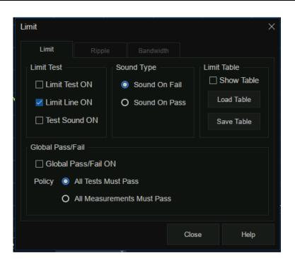
Figure 8-6 Limit test interface
