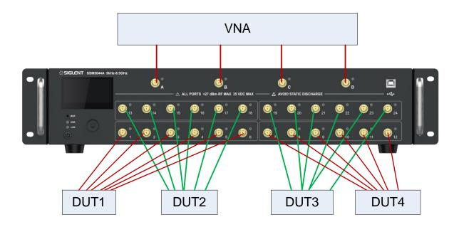
VNA and switch matrix combined expansion port diagram
