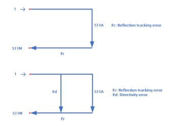
Figure 7-6 Schematic diagram
