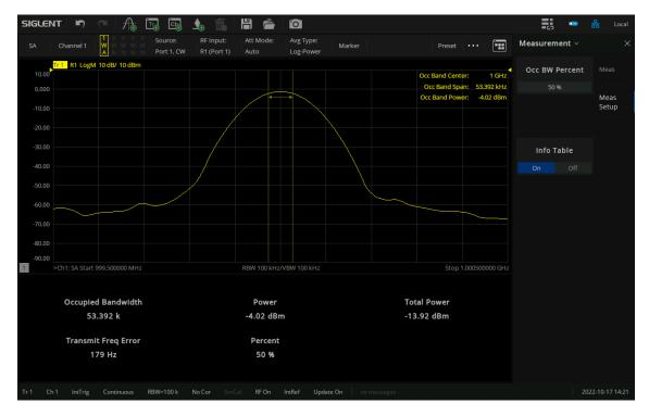
Figure 11-15 Occupied BW measurement
