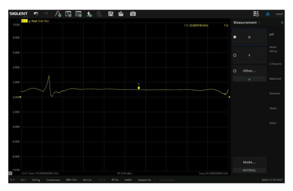
Figure 15-16 Permeability Measurement Results (PEI Material)
