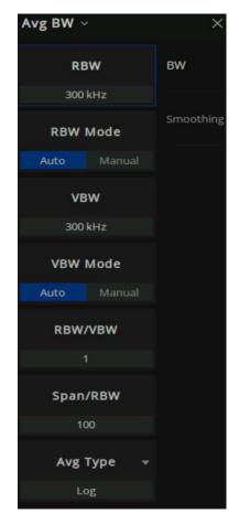
Figure 11-5 Spectrum analysis signal processing setup menu
