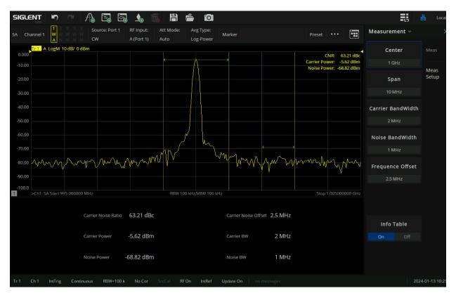
Figure 11-17 CNR measurement
