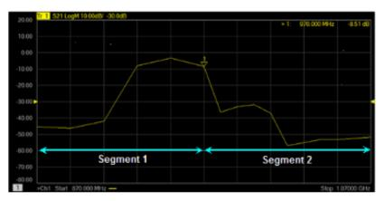
Figure 6-2 X-point spacing is not used
