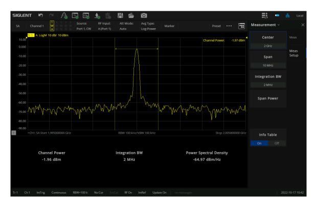
Figure 11-13 Channel Power measure
