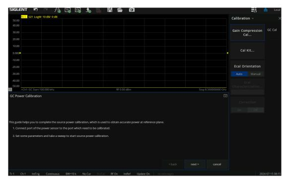
Press [Cal] > Gain Compression Cal... to enter the calibration wizard.
