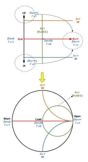
Figure 6-5 Schematic diagram of Smith circle
