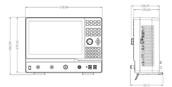
Figure 5-1 Front view and side view
