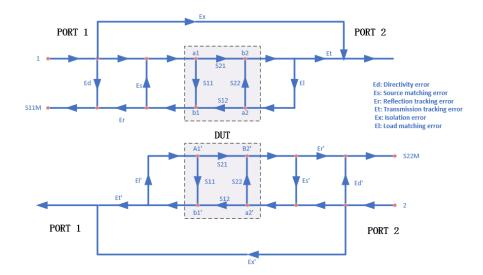
Figure 7-9 Error model diagram
