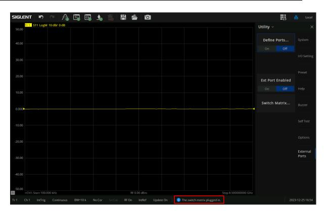
Press the System >"External Ports" >"Ext Port Enabled" to enable the function, then the matrix identifier is displayed on the upper right corner of the UI.
