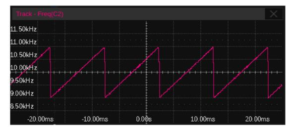
The upper limit of the statistic number in a frame is set in <u>Statistics</u> > <u>AIM Limit</u>, which means the values exceeding the limit will not be shown in the track plot. The upper limit is 1,000 by default and can be set to up to 100,000.
