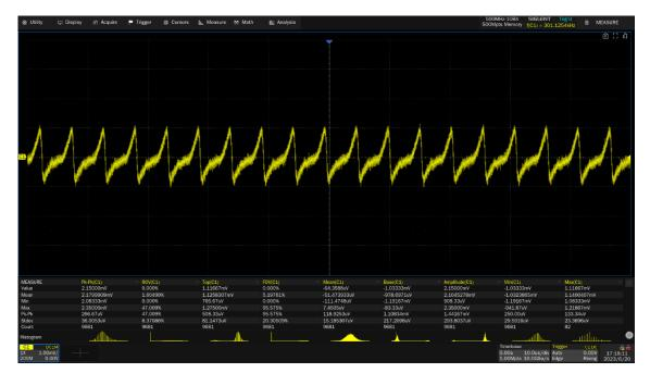
In M2 mode, up to 12 parameter measurements are displayed at a time. When statistics are enabled, they are distributed on the right side of the measurement item. Click a row to add or replace a measurement.
