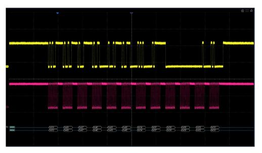
If the data width is set to be greater than 8 bits (such as 16 bits), measure the clock idle time between 8-bit data packets as 2.5 us, and then set the timeout time to a value between 2.5 and 30 us. In this example, it is set to 5 us:
