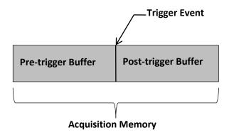
Below is the definition of the states in the process of filling the acquisition memory:
