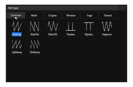
There are 6 tabs in the window. Under each tab, a catalog of waveforms is listed. Built-in waveforms are stored in Common, Math, Engine, Window, and Trigo. Stored waveforms are located in the Stored menu.
