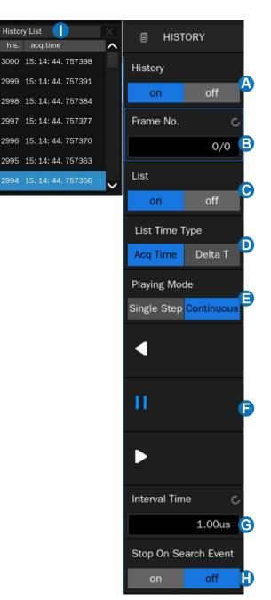
The oscilloscope automatically stores acquired frames. It can store up to 124,000 frames but the number may vary due to the memory depth and timebase settings. Turn on history mode, then the stored frames can be recalled and measured.
