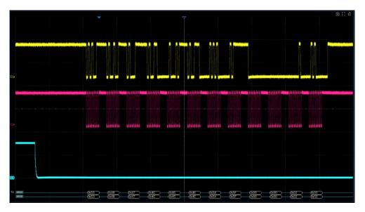
When the CS type is set to Clock Timeout, turn on Cursor, measure the clock idle time between frames as 0.3 us, and measure the interval between clock pulses as 30 us, then set the timeout to a value between 0.3 us and 30 us. In this example it is set to 1 us:
