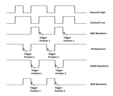
Logic (AND, OR, NAND, NOR), source, limit range, and time value can be set in the trigger dialog box.
