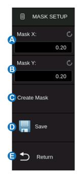
Under mask testing, the user detects signal changes by creating specific rules for the signal to be detected (including setting the horizontal and vertical adjustment range of the signal), and then observing whether the signal is outside the rule range.
