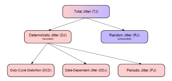
Figure 33.1 Jitter decomposition tree
