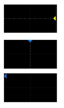
**Trigger Level Indicator** shows the level where the waveform triggers on the vertical axis.
