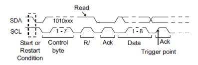
7 Address & Data -- the oscilloscope will be triggered on the read or write frame in 7-bit address mode.
