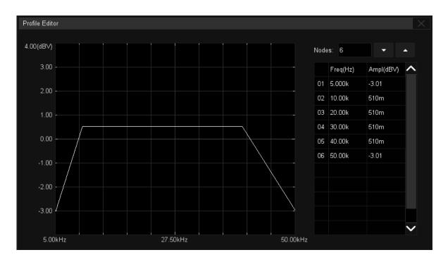
Click *Nodes* to set the signal node number through the mouse wheel, or click  $\blacktriangle$  to increase the nodes and  $\checkmark$  to decrease.
