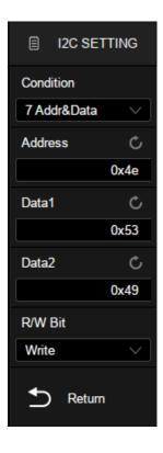
**Data Length** -- The data length range is 1 to 12 bytes. When the SDA data length is equal to the value of Data Length and address length is the same as the set value, the oscilloscope will be triggered.
