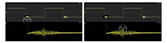
Adjust the horizontal scale of Zoom window by horizontal pinch and spread in the zoom area of the main window or the Zoom window.
