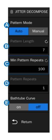
The result of jitter decomposition will be shown in the measured area. Users can add the jitter components interested, including measurement values, histogram, track, and spectrogram. Refer to the "Jitter Measure" section for details.
