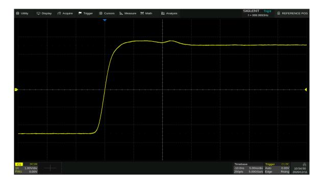
Fixed position, timebase is changed to 5 ns/div, the grid number of delay (-2div) remains fixed, while the horizontal delay changes to -10 ns
