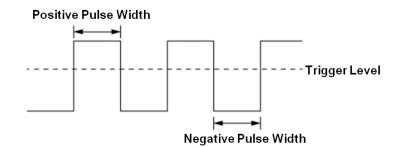
Less than a time value ( $\leq$ ) -- Trigger when the positive or negative pulse time of the input signal is lower than the specified time value. Below is an example of a trigger condition set to a positive pulse width < 100ns
