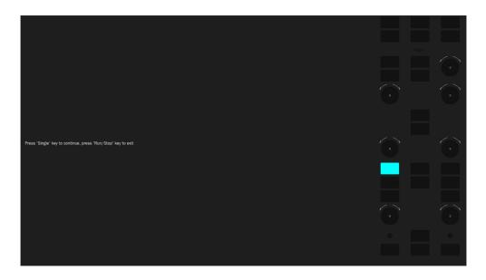
Press Single button and the first LED on the front panel will light. The corresponding position of the key on the screen will also change color. Press the Single button to check the next button.
