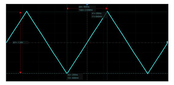
X+Y (horizontal + vertical) -- Both the X cursors and Y cursors are enabled.
