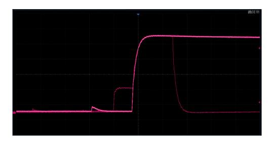
In this case zone trigger is a quick and simple way to capture the waveform. Enable the zone trigger, and draw a box to intersect with the bus contention part, as shown in the figure below:
