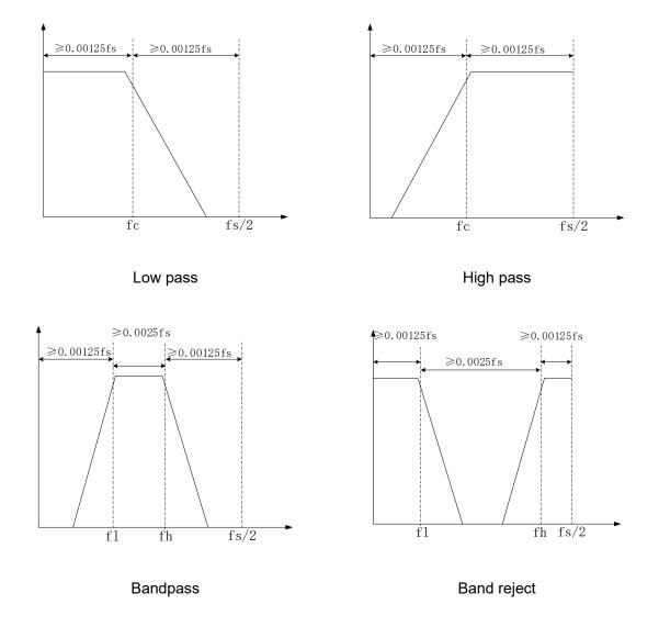
Take a Low pass filter as an example. It requires that the corner frequency (fc) is not less than 0.00125\*fs (i.e. fc  $\ge 0.00125$ \*fs), and the 0.00125\*fs wide roll-off does not exceed the 1st Nyquist zone (i.e. (fs/2) - fc  $\ge 0.00125$ fs). If fs = 20 GSa/s, then the legal range of the corner frequency (fc) is 25 MHz~9.975 GHz
