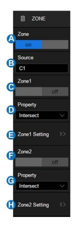
The zones can be created and moved by the mouse or by setting *Zone Setting* in the dialog box. The color of the zone's outline is consistent with the color of the specified source (Channel 1 = Yellow, etc...).
