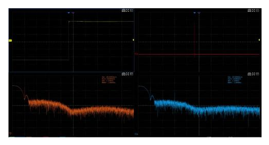
This example uses two nested operations to achieve FFT analysis of the differential operation results of C1 waveform:
