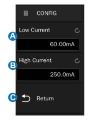
**Note:** The low and high current values are used to calculate the trigger level and adjust the oscilloscope vertical scale. After the load changes, the current value changes from low to high (or from high to low), and the oscilloscope triggers and performs to measure the transient response stability time.
