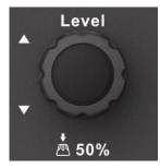
All the knobs on the front panel are multi-function. They can be pushed as well as rotated. Pushing a knob quickly recalls a specific function, which is indicated by the silkscreen near the knob.
