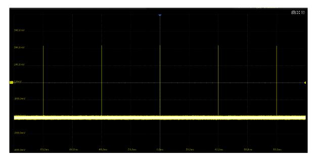
In normal mode, 5 pulses can be obtained on the screen with the sample rate of 500MSa/s at 100Mpts memory depth.
