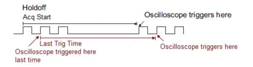
Acq Start -- The initial position of holdoff is the first-time point satisfying the trigger condition. In the example above, each holdoff starts from the first rising edge of the pulse sequence.
