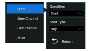
**Start** -- The oscilloscope will be triggered at the start of the message (after 56 Sync ticks). You can select the type of message: Fast Channel Message, Slow Channel Message, or any.
