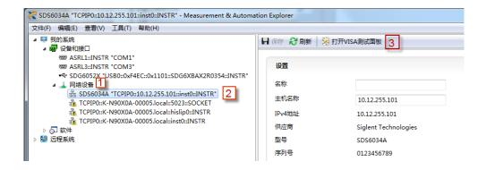
5. Click "Open VISA Test Panel "option button, which then displays the following interface (below). Then click the "Input/Output" option button and click the "Query" option button. The "Read" operation information will be displayed.
