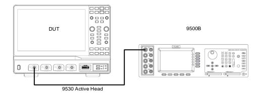
Figure 7 Test setup for DCG / Offset / Timebase...
