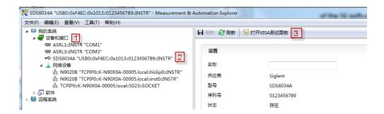
4. Click "Open VISA Test Panel" option button, and then the following Interface will appear. Next, click the "Input/Output" option button and click the "Query" option button to view the Read operation information.
