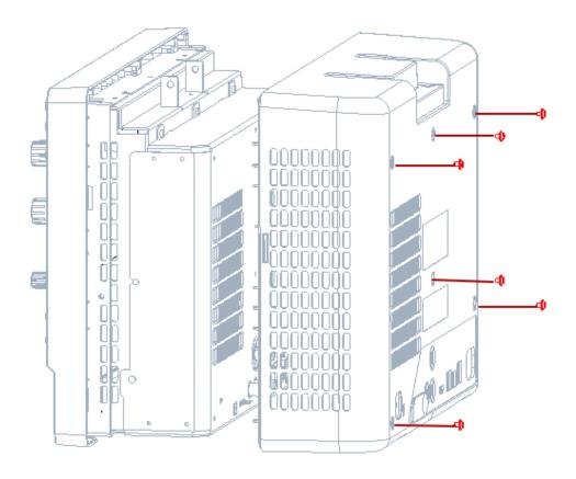
Figure 12 To remove the rear cover
