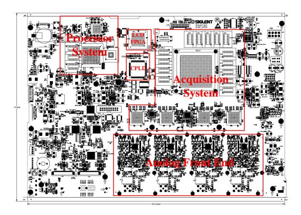
Most of the test points are located on the top side of the board, it is not necessary to completely remove the board from the chassis to do the troubleshooting unless noticed. It is recommended to re-assemble the power supply module to the metal frame for safety considerations. Follow the instructions in chapter **Disassembly Procedures**.
