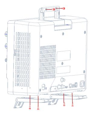
Figure 11 To remove the handle and foot
