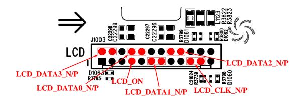
Figure 25 Test points for LCD signal
