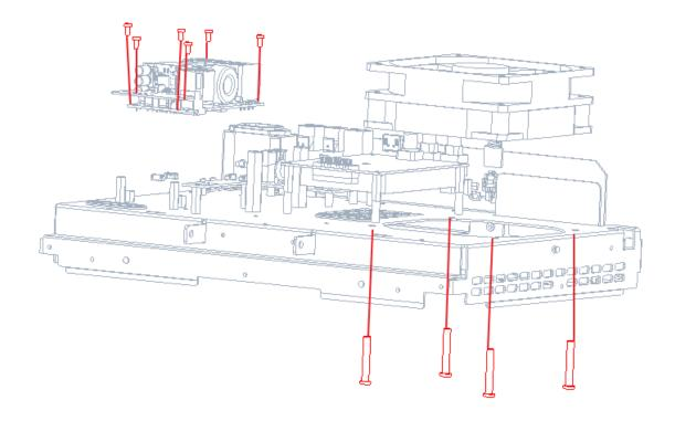
Figure 15 To remove the power supply module and fan.
