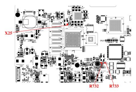
Figure 22 Test points for clock
