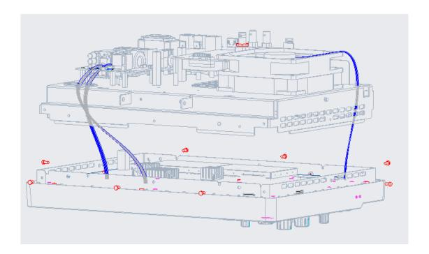
Figure 14 To remove the back panel chassis module.
