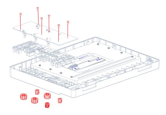
Figure 17 To remove the rubber keypad and keyboard
