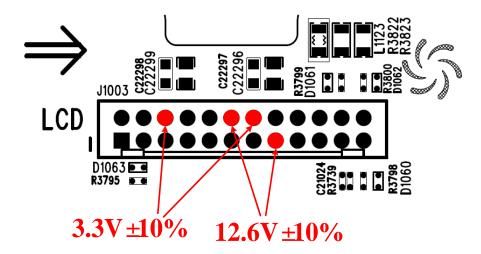
Figure 24 Test points for the LCD power supplies
