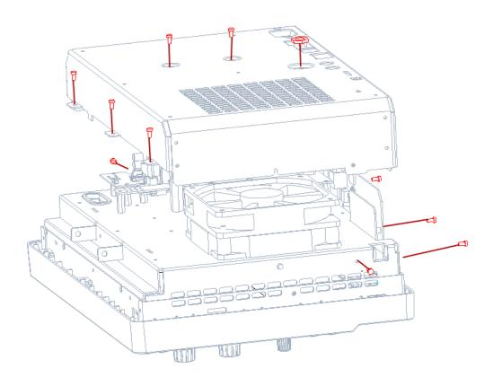
Figure 13 To remove the rear metal cover
