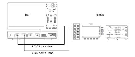
Figure 8 Test setup for Channel skew
