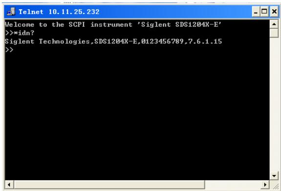
6. To exit the SCPI> session, press the Ctrl+] keys simultaneously.
