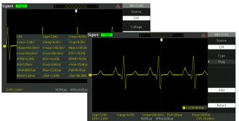
The SDS1000DL+/CML+ support voltage, time and delay measurement types, with a total of 32 different parameters. The user is able to select five measurements to display on the screen. All measurement parameters can also be displayed simultaneously.
