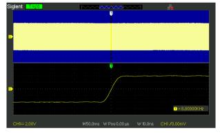
Zoom can extend a partial segment of the waveform, giving the user not only an overview of the whole signal but also a detailed view of the zoomed-in segment. The Zoom feature is a convenient way to locate a specific segment of a signal while zooming in to see the details.
