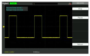
The digital recorder is able to record data in real-time and without any dead time. SDS1000DL+/CML+ supply 7 M of memory for the recorder and support a USB disk.
