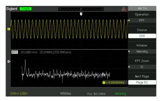
SDS1000DL+/CML+ provides 5 kinds of math operation: +, -, \*, /, FFT, supporting channel waveform and FFT waveform in either split display windows or both signals appearing on the full screen.
