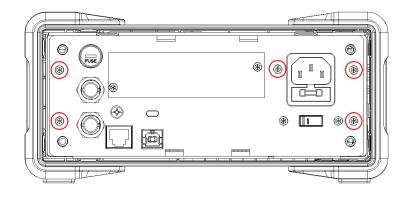
7. Unscrew the 4 screws and remove the fan.
