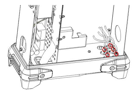
9. Remove the cable and unscrew all the screws,then you can remove the PCBA.
