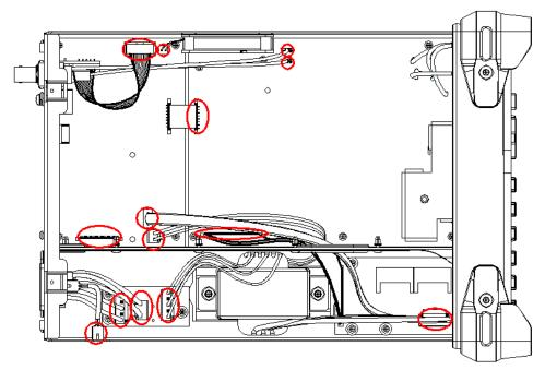
6. Unscrew the 5 captive screws in the rear metal cover and remove the rear metal cover.
