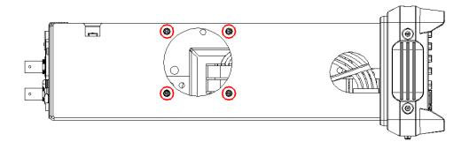
8. Remove the cable plug connected to the front pannel.
