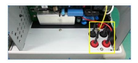
9. Remove the cable and unscrew all the screws,then you can remove the PCBA.
