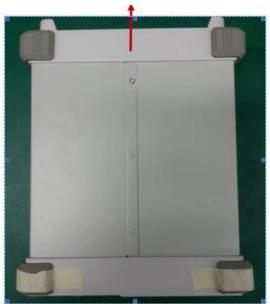
4. Remove the screw on the bottom of the instrument and place it in a safe location for re-assembly. Slide off the instrument cover as indicated by the arrow shown below.
