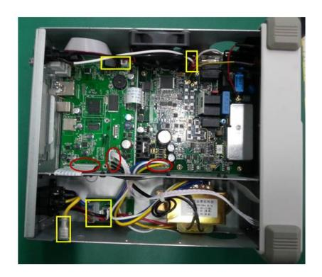
6. Unscrew the 5 captive screws in the rear metal cover and remove the rear metal cover.
