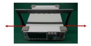
3. Unscrew the two captive screws in the rear bezel and remove the rear bezel as indicated by the arrow shown below
