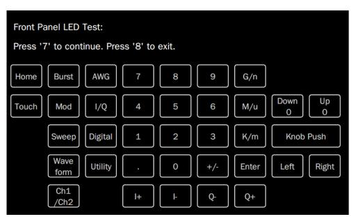
Press the 7 button and the first LED on the front panel will light. The corresponding position of the key on the screen will also change color. Press the 7 button to check the next button. Press the 7 button consecutively until all the backlights are tested.
