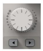
In addition to directly typing parameter values with the numeric keypad, you can also use the knob for continuous adjustment of parameters.
