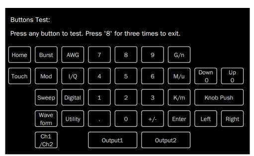
Knob test: Turn the knob clockwise, counter-clockwise, and press down. Observe whether the value on the corresponding knob (default 0) on the screen increases or decreases in real-time and whether the knob lights up when it is pressed.
