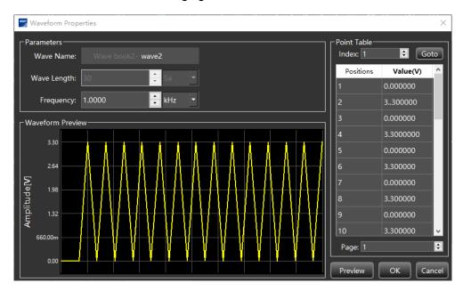
4. The waveform generated can be previewed in the waveform preview window. Select "Display Properties "in the "Property" area of the toolbar, and change the "Interpolation" to "0-order hold", to obtain the correct waveform preview of the digital clock:
