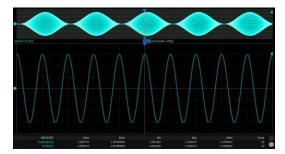
100% modulation depth time-domain diagram
