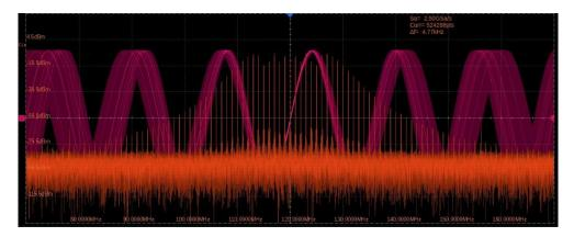
Frequency measurements were taken on the modulated signal and the frequency versus time (Tracking diagram) was plotted as below, reflecting the frequency versus modulating shape characteristics of the modulated waveform.
