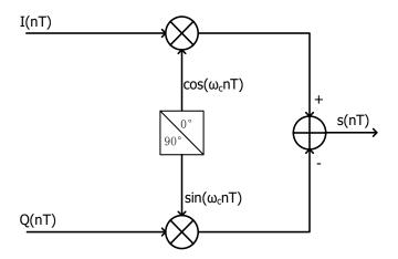
Figure 9-6 Schematic block diagram of quadrature modulator
