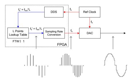
Figure 9-2 Principle block diagram of TrueArb Technology
