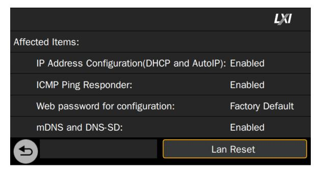
Touch *LAN Reset* to restore the LAN defaults to your oscilloscope. It will enable automatic IP, ICMP Ping responder, and Multicast DNS, and reset the webserver
