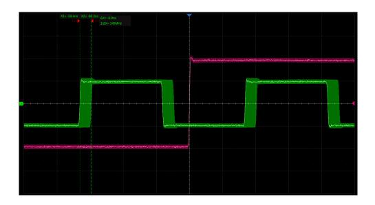
As we can see from the table above, the frequency errors introduced on both channels are small, but not proportional, which results in the two frequencies that were integer multiples no longer being integer multiples, with the result that they are not phase-locked. The following is the phase drift (approximately 6.9 ns) observed in this example after 17.3 hours for both channels in "Independent" mode.
