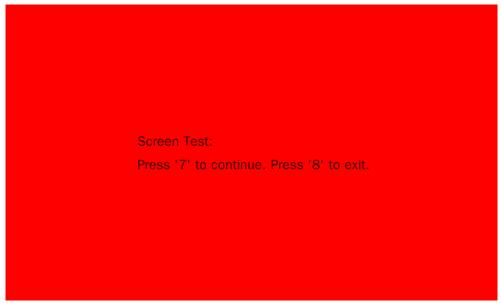
Press 7 to switch to green and blue screen display mode. Observe whether there is any color distortion, bad pixel or scratch on the screen.
