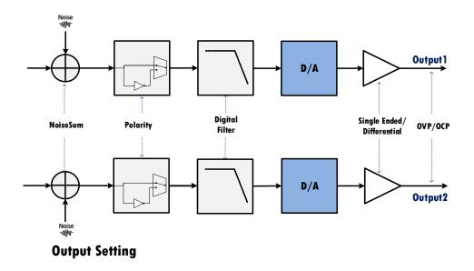
Figure 13-1 Block diagram of output setting
