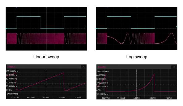
This example will help the users to better understand the difference between a linear sweep and a logarithmic sweep: scanning from 100 Hz to 100 kHz with a sweep time of 3 ms increases the frequency by a factor of 10<sup>3</sup> and by a factor of 10 for every 1 ms in a logarithmic sweep. The table below shows the frequency values corresponding to each time point in logarithmic and linear sweep mode.
