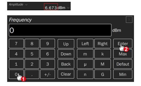
Set offset: Click the parameter value area of offset in the "Offset" parameter setting box, and then type 0 and Enter in sequence in the pop-up virtual keyboard.
