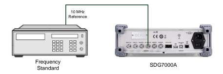
Figure 17-2 time base calibration environment
