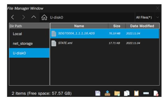
Select the correct ads file in the file manager and select to start the upgrade. The device first copies the upgrade file (\*.ads) to the local memory and parses it. If the parse succeeds, it will upgrade. After the updating is finished, the generator will restart automatically.
