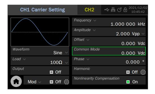
Note the distinction between the concepts of "Common Mode" and "Offset". Both are DC levels, but "Common Mode" refers to the common-mode component of the differential pair, while "Offset" is the differential mode component.
