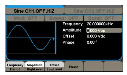
**Note:** You can also enter the desired value using the knob and direction keys.
