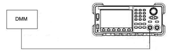
3. Select Sine waveform of the generator and set the amplitude to the values listed below in sequence.
