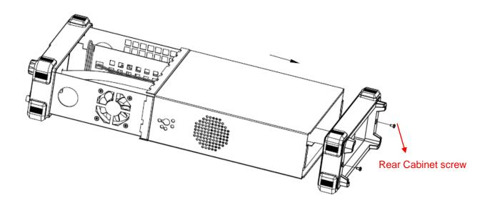
Table 4-3 Removing the Metal Shell and Rear Cabinet
