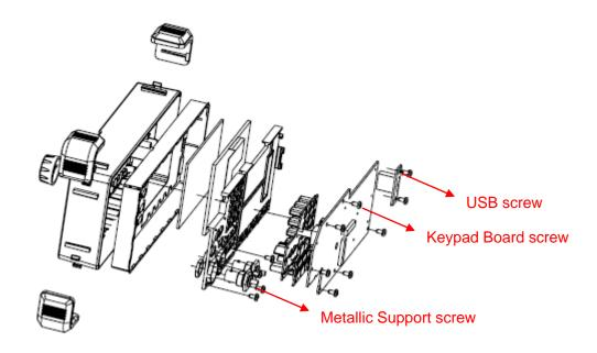
Table 4-5 Removing the display module screws
