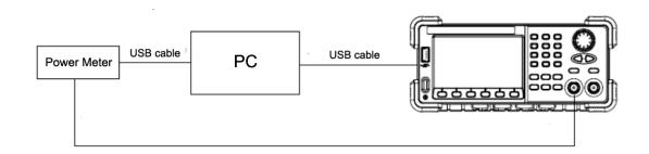
3. Select Sine waveform of the generator and set the amplitude to 1 V, and then step through the frequencies listed below in sequence. Then, set the amplitude to 2.5V and repeat the frequency steps.
