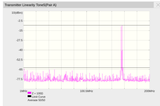
Figure 7-9 Tone1 Example of Transmitter Linearity Results
