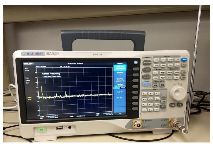
2. Press Frequency > Center Frequency and set the center frequency to match the frequency of interest. Here, we are setting the center frequency to 100.7 MHz, a local FM radio station:
