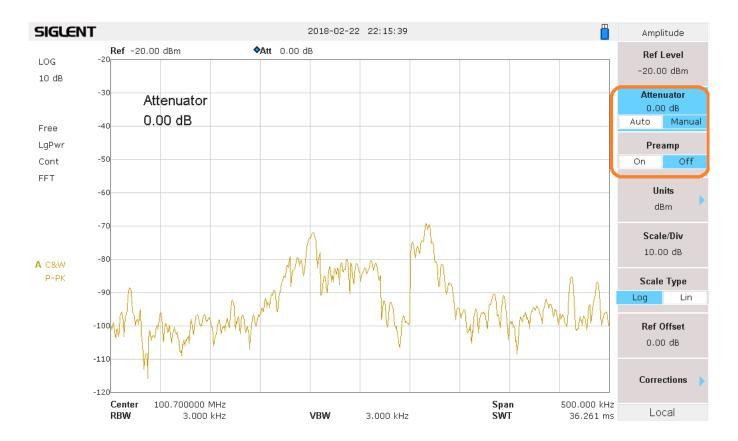
After adjusting the preamp and attenuator, you can see the signal rise out of the noise:
