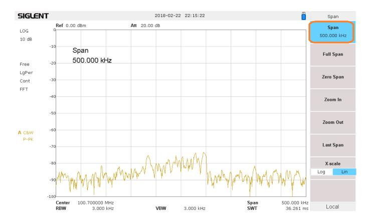
3. If the signal is still very low or cannot be easily observed through the noise, you can lower the attenuation by pressing Amplitude > and lower the Attenuator setting. You can also enable the preamplifier.
