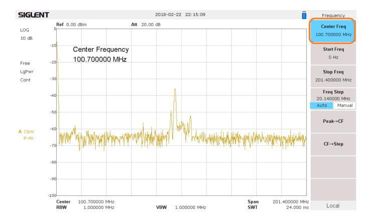
2. Press Span > Span and set the span to an appropriate level for your application. If you are looking at a single channel, you can set the span to 500 kHz or so. This will allow you to observe the channel and the full range of the frequency deviation:
