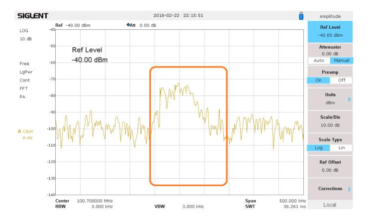
4. Now, we can activate another trace on the display and we can set it to be a Max Hold trace type. This trace type records the largest amplitude for each frequency bin and it will stay there until it has been manually cleared. Over time and successive scans, the Max Hold trace will show us the frequency deviation of our signal.
