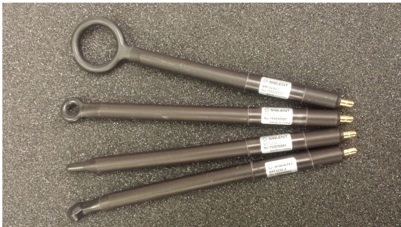
Figure 5: SIGLENT SRF5030 near-field probe kit.
